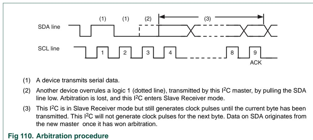
The synchronization logic will synchronize the serial clock generator with the clock pulses on the SCL line from another device. If two or more master devices generate clock pulses, the “mark” duration is determined by the device that generates the shortest “marks,” and the “space” duration is determined by the device that generates the longest “spaces”.
