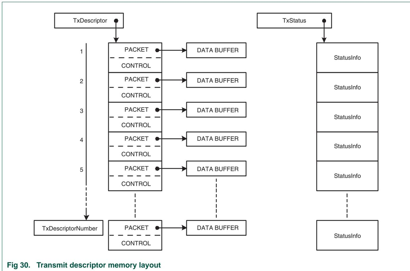
Fig 30. Transmit descriptor memory layout
