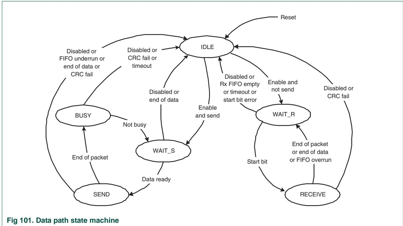
Fig 101. Data path state machine
