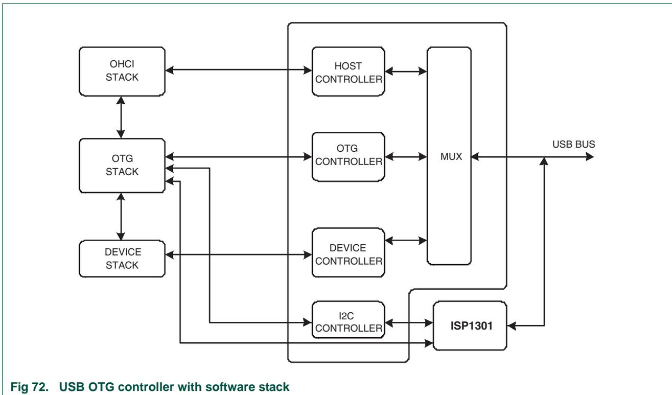
Fig 72. USB OTG controller with software stack
