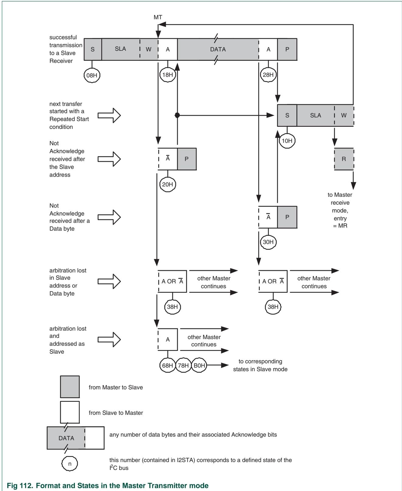
Fig 112. Format and States in the Master Transmitter mode
