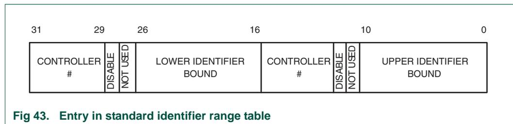
**Fig 43. Entry in standard identifier range table**
