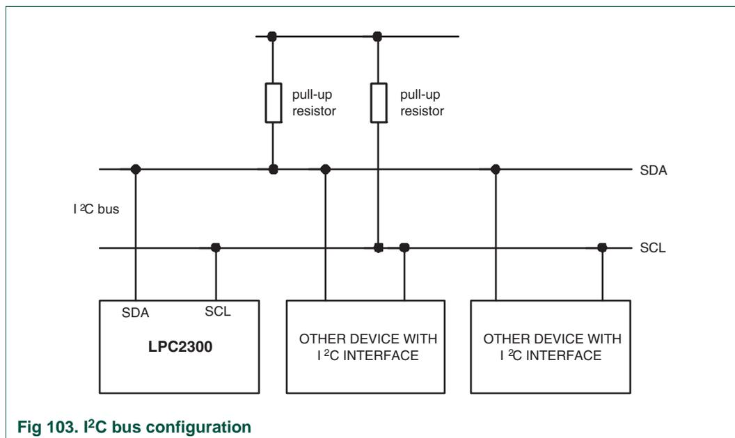
Fig 103. I<sup>2</sup>C bus configuration
