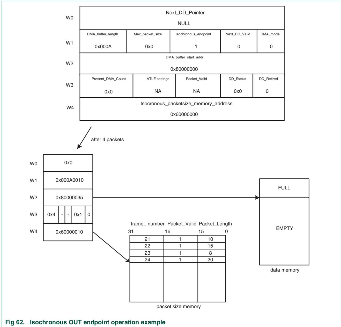
Fig 62. Isochronous OUT endpoint operation example
