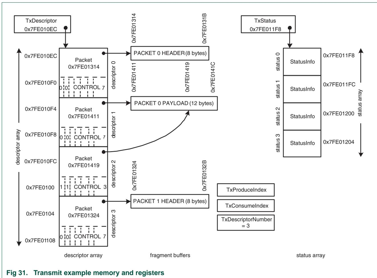
**Fig 31. Transmit example memory and registers**
