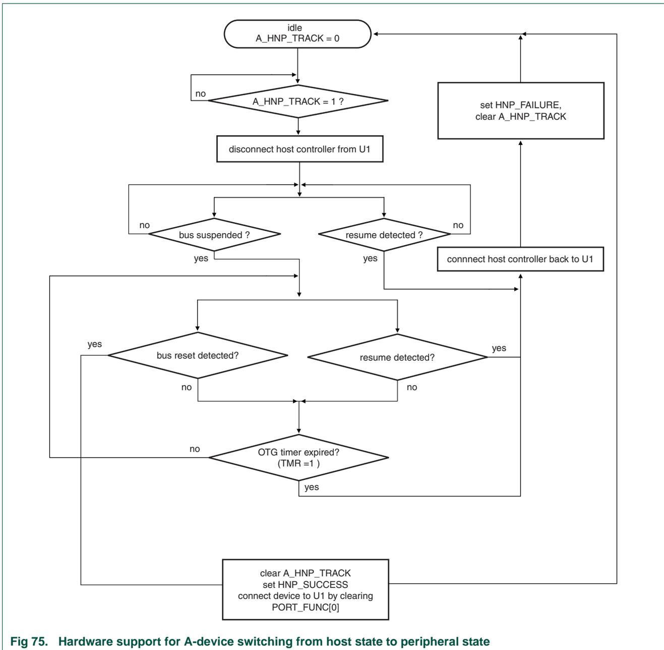
Fig 75. Hardware support for A-device switching from host state to peripheral state
