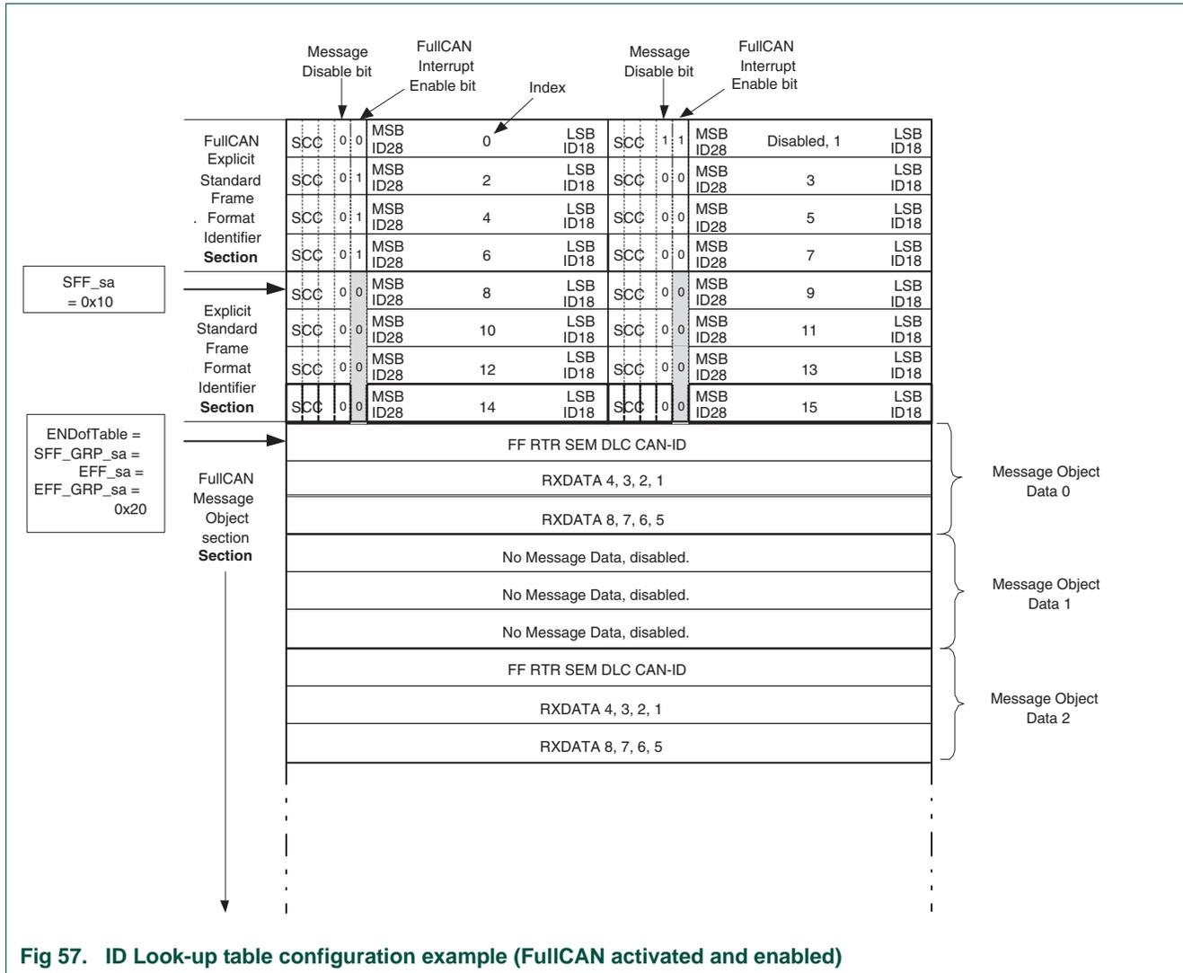
Fig 57. ID Look-up table configuration example (FullCAN activated and enabled)
