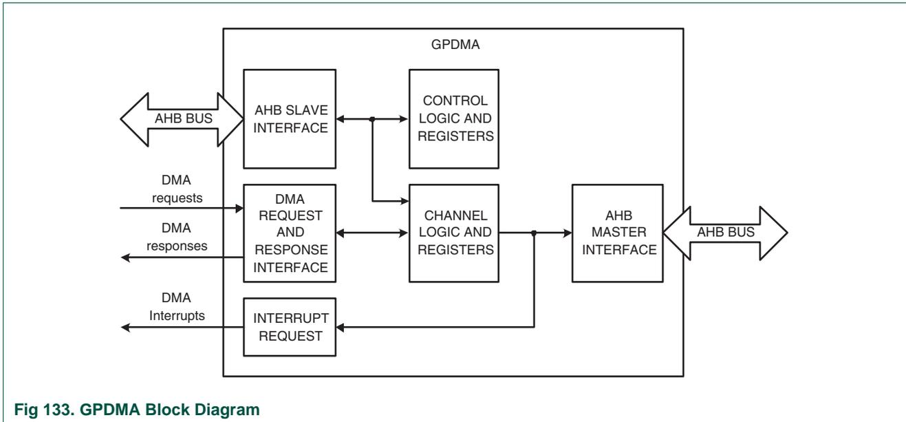
**Fig 133. GPDMA Block Diagram**
