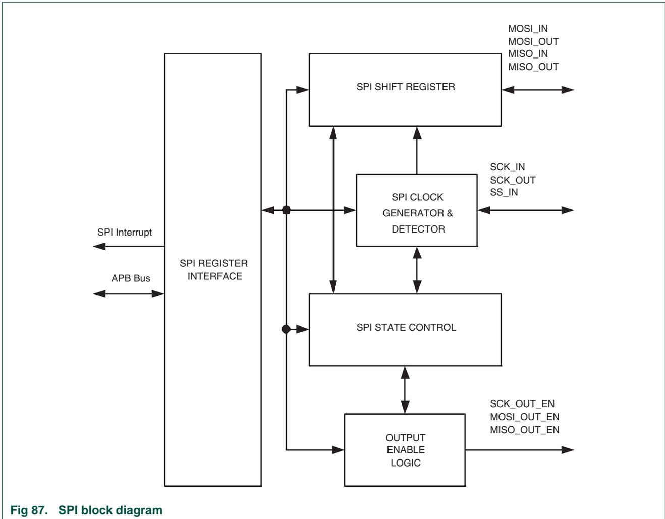
Fig 87. SPI block diagram
