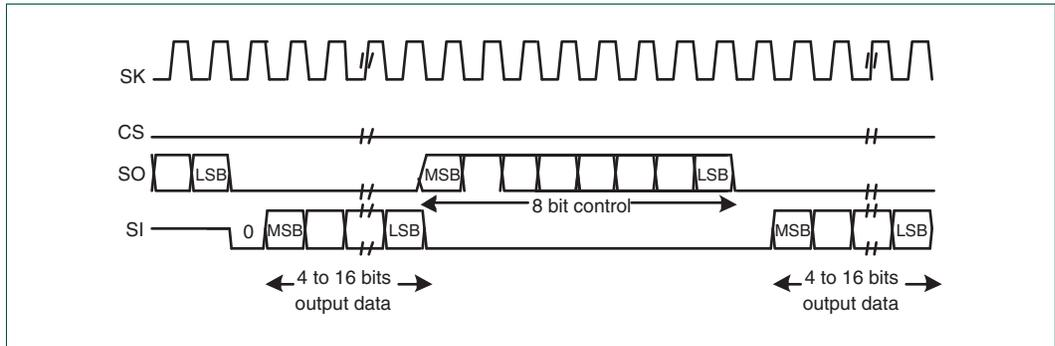
Fig 94. Microwire Frame Format (Continuous Transfers)
