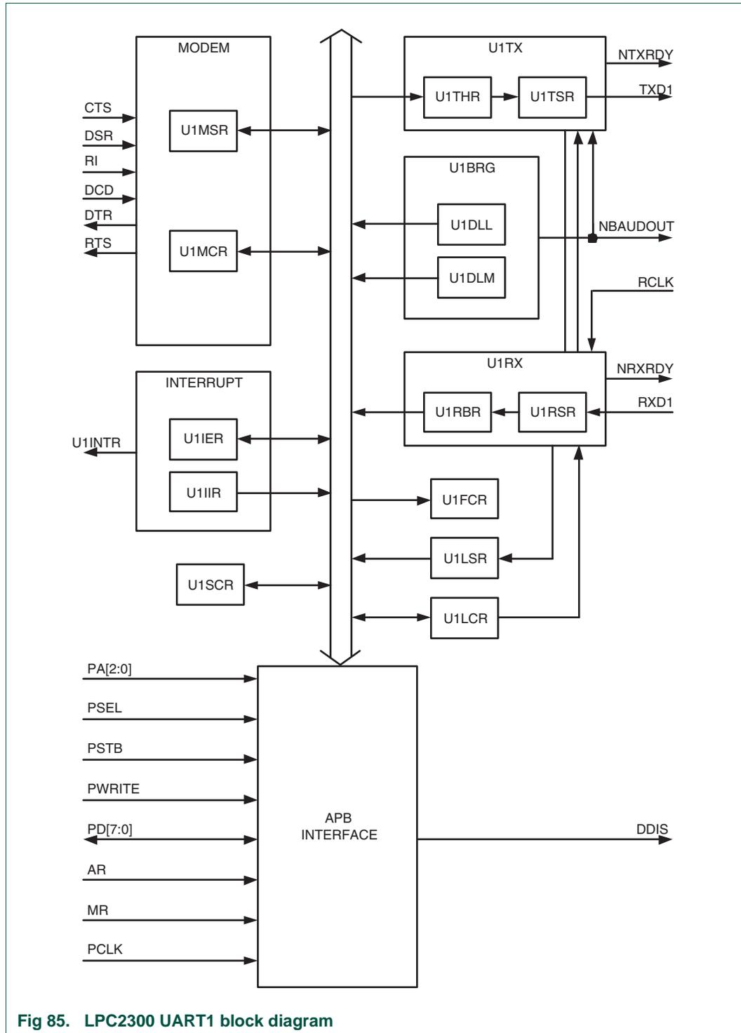
Fig 85. LPC2300 UART1 block diagram
