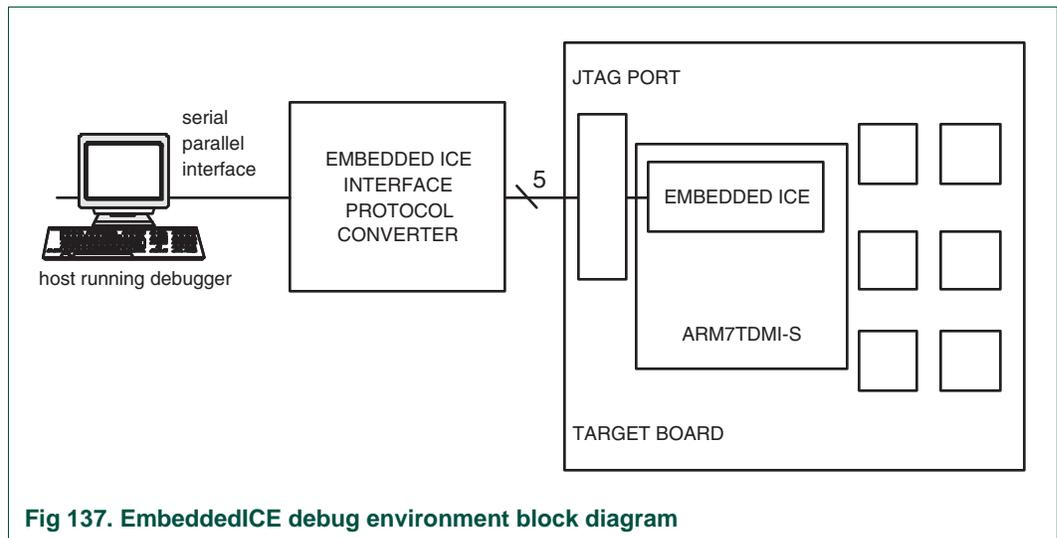
Fig 137. EmbeddedICE debug environment block diagram
