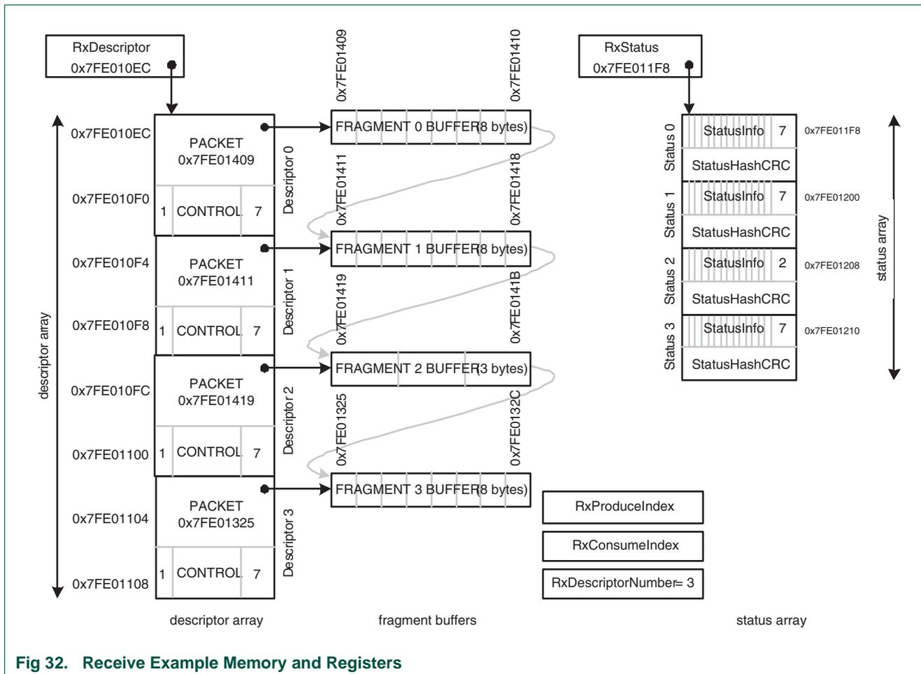
Fig 32. Receive Example Memory and Registers
