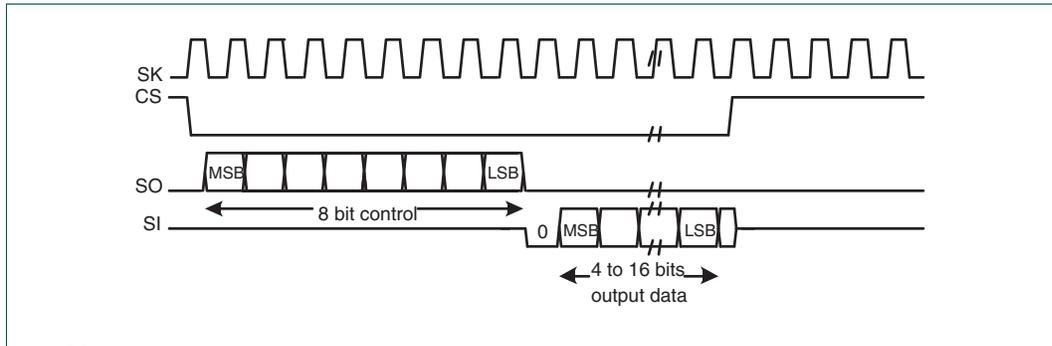
**Fig 93. Microwire Frame Format (Single Transfer)**
