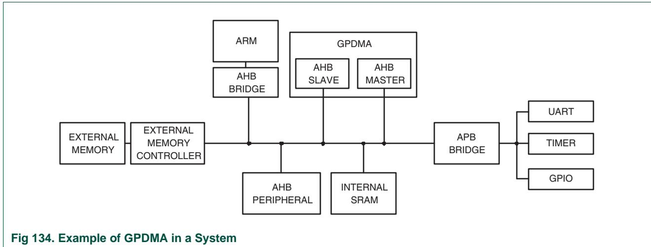
**Fig 134. Example of GPDMA in a System**
