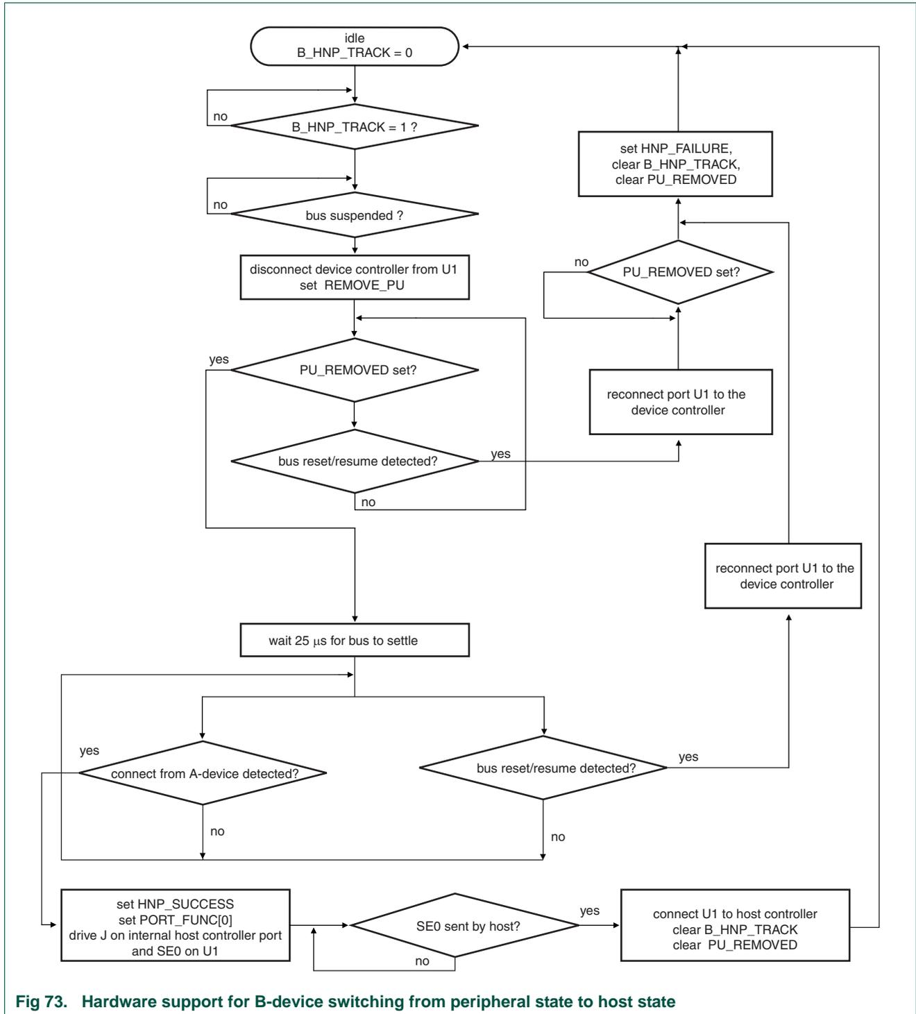
Fig 73. Hardware support for B-device switching from peripheral state to host state
