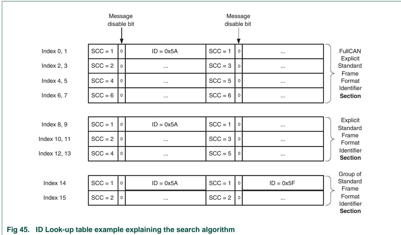
The identifier 0x5A of the CAN Controller 1 with the Source CAN Channel SCC = 1, is defined in all three sections. With this configuration incoming CAN messages on CAN Controller 1 with a 0x5A identifier will find a match in the FullCAN section.
