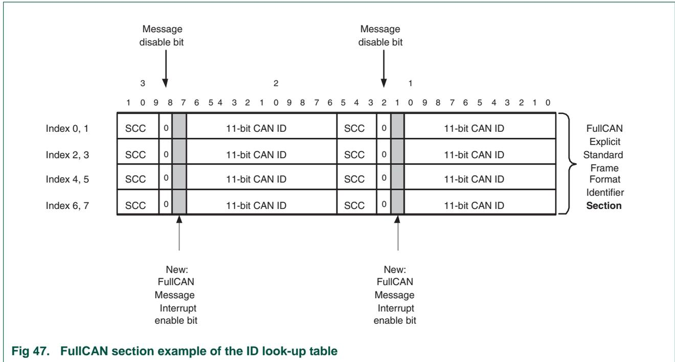
Fig 47. FullCAN section example of the ID look-up table
