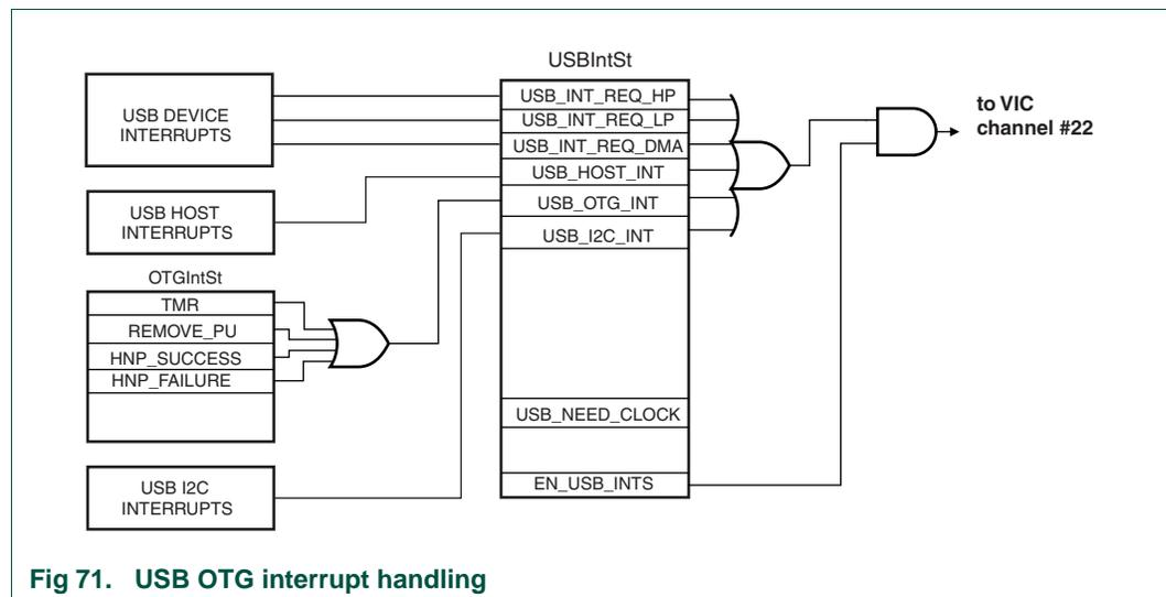
**Fig 71. USB OTG interrupt handling**
