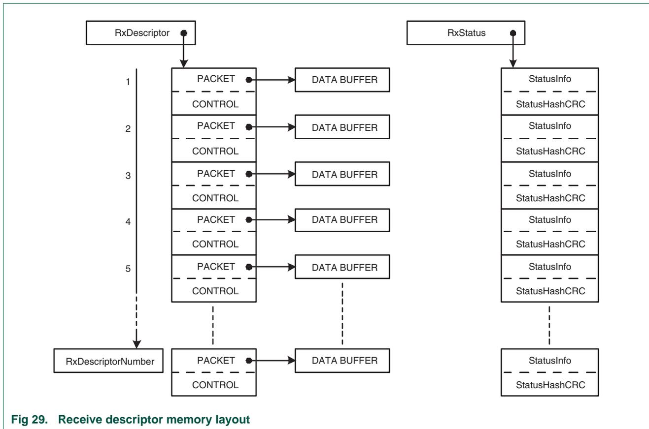
Fig 29. Receive descriptor memory layout
