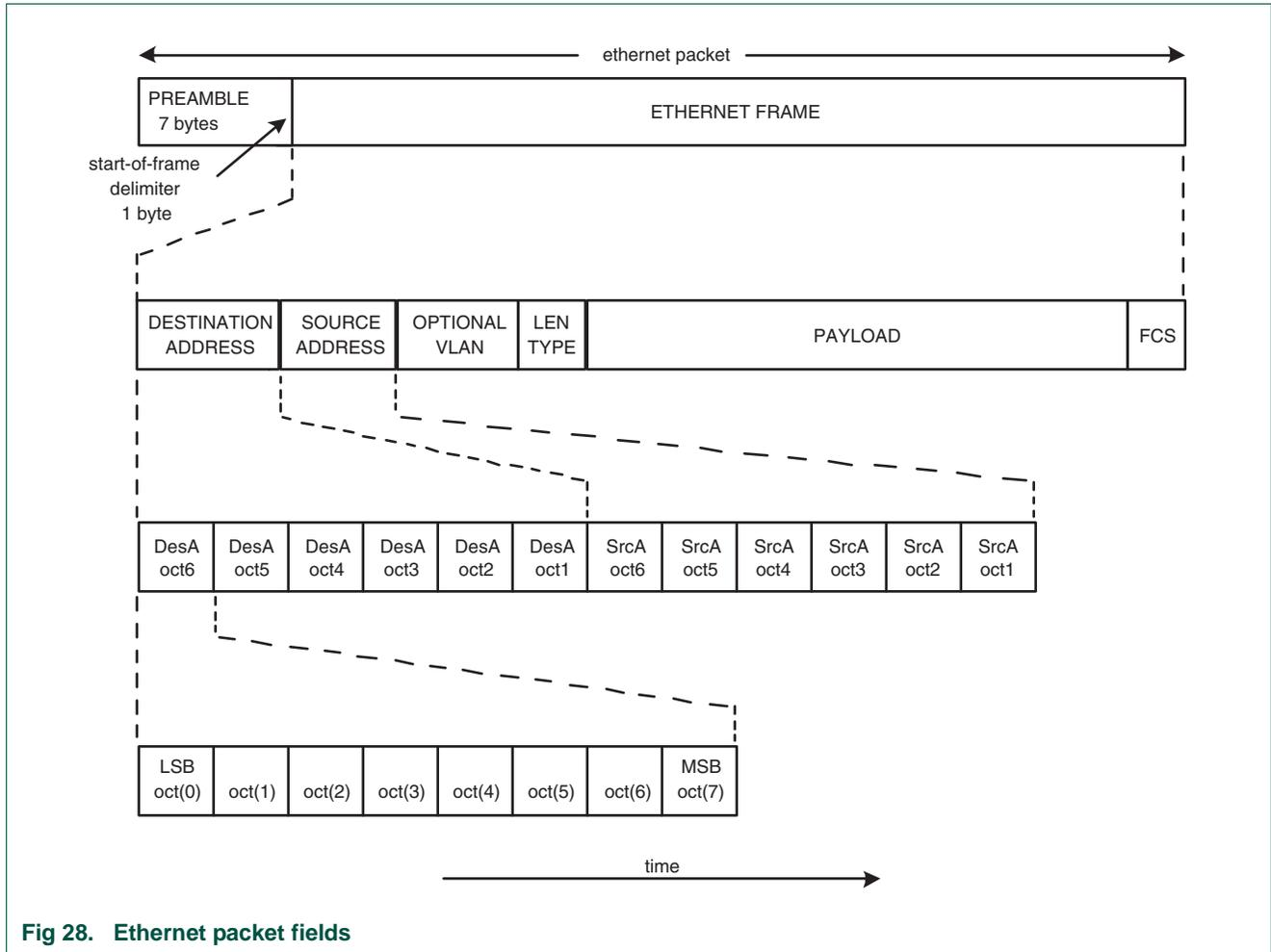
Fig 28. Ethernet packet fields
