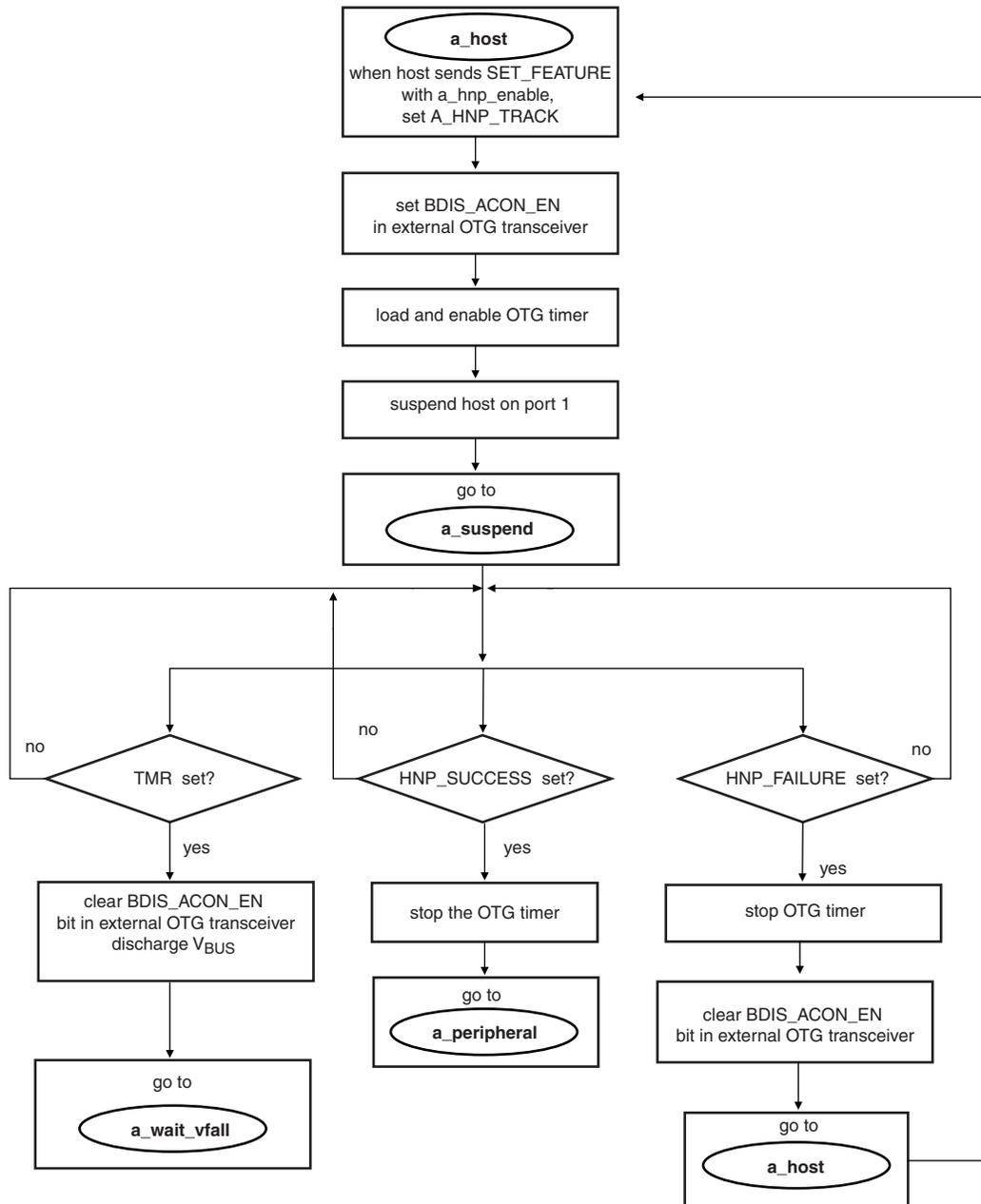
Fig 76. State transitions implemented in software during A-device switching from host to peripheral
