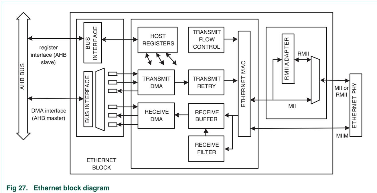
Fig 27. Ethernet block diagram
