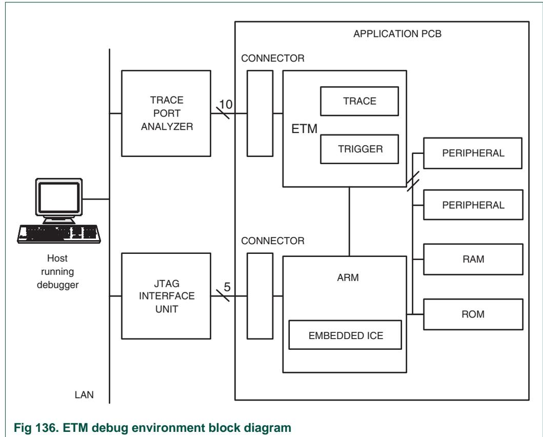
Fig 136. ETM debug environment block diagram
