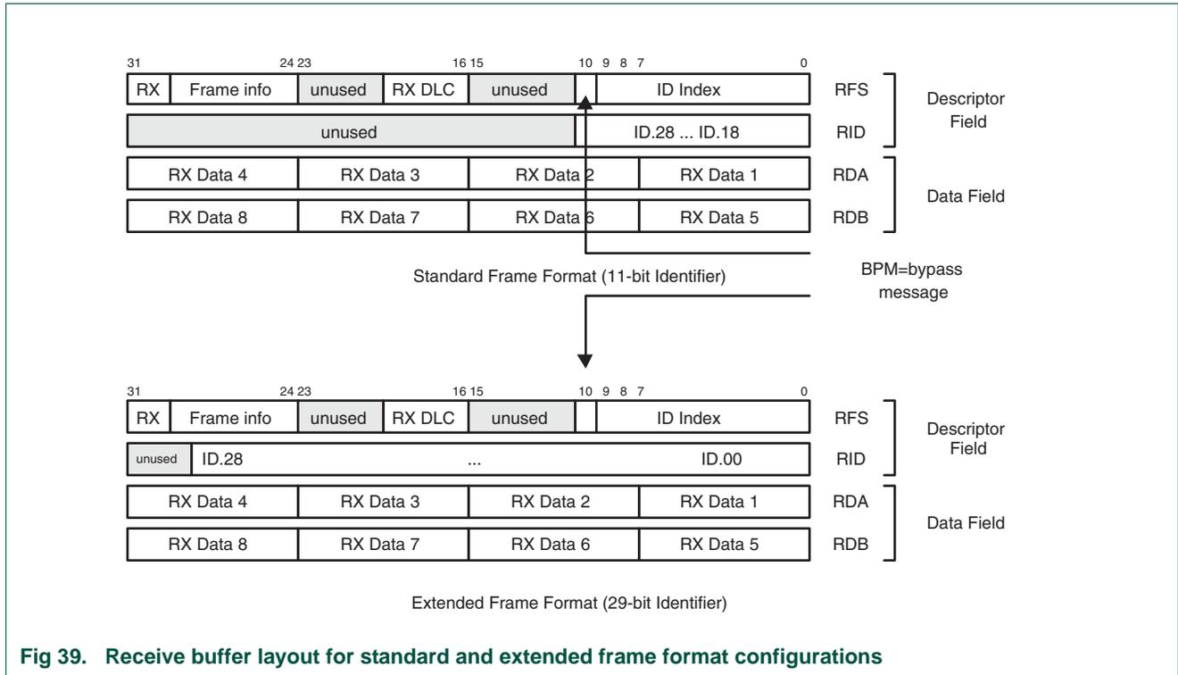
Fig 39. Receive buffer layout for standard and extended frame format configurations
