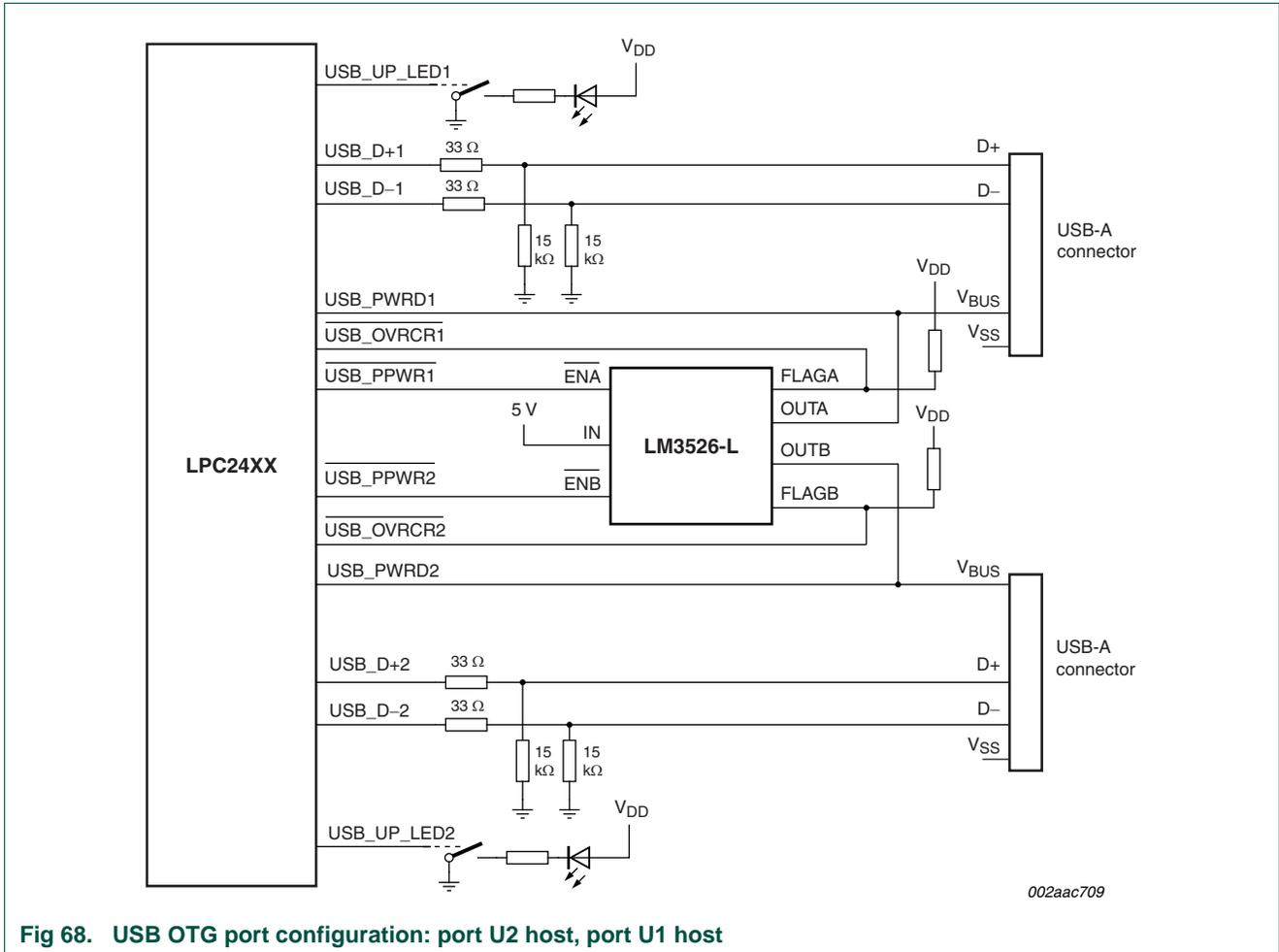
Fig 68. USB OTG port configuration: port U2 host, port U1 host
