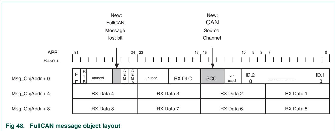
Fig 48. FullCAN message object layout
