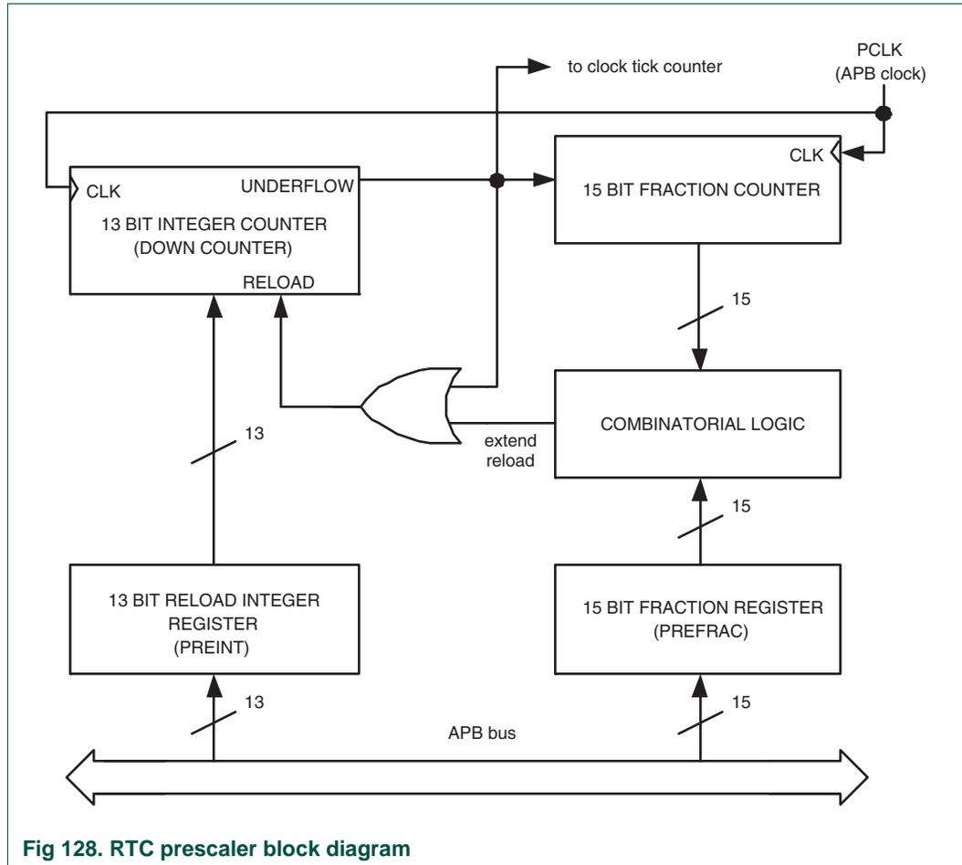
Fig 128. RTC prescaler block diagram
