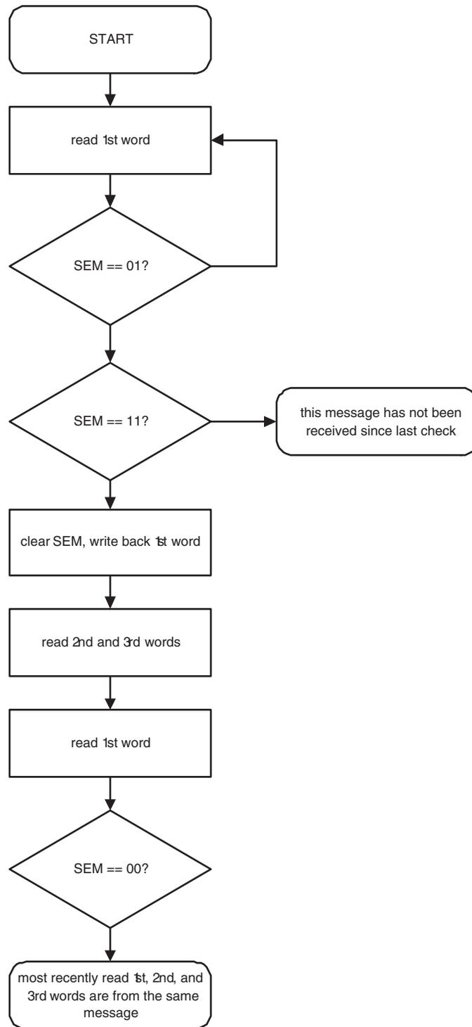
Fig 46. Semaphore procedure for reading an auto-stored message
