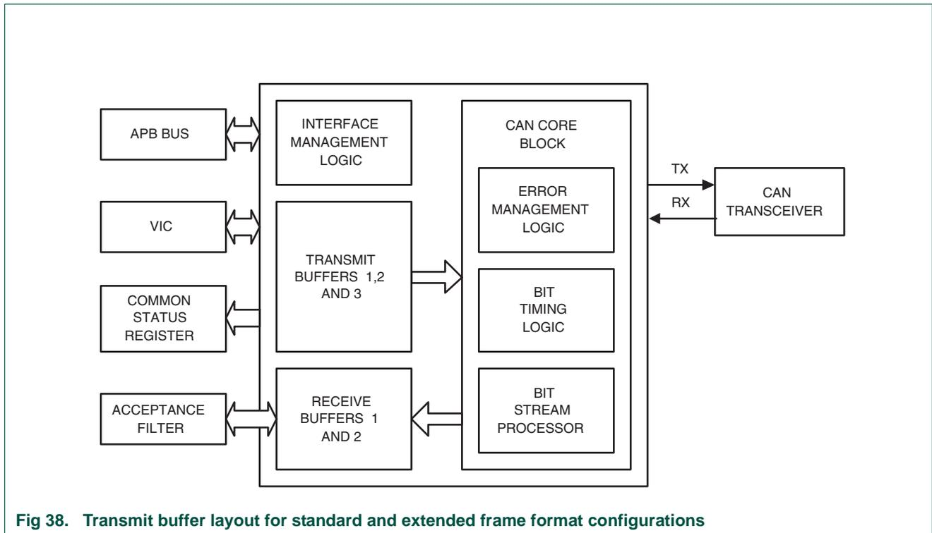
Fig 38. Transmit buffer layout for standard and extended frame format configurations
