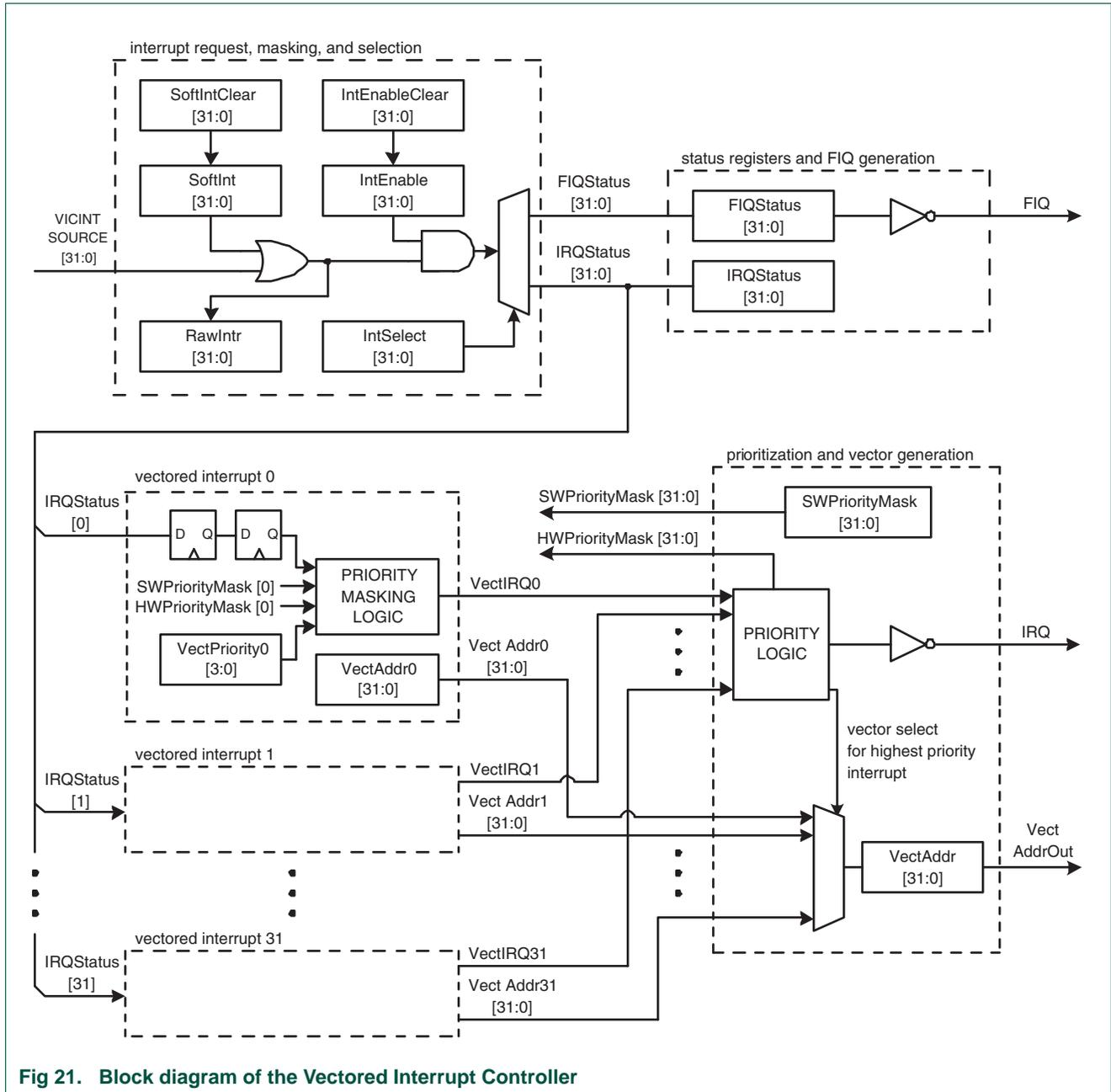
Fig 21. Block diagram of the Vectored Interrupt Controller
