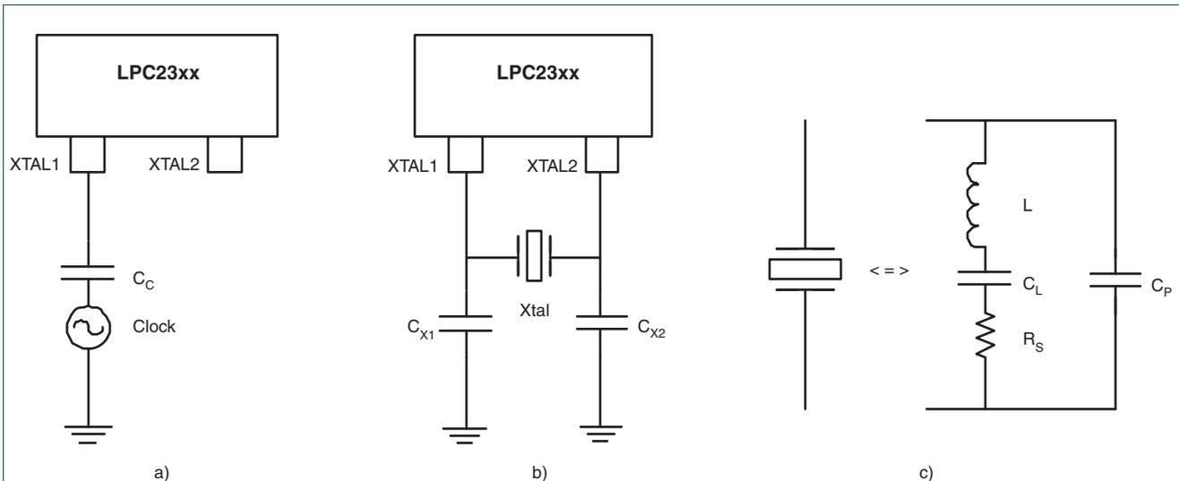
**Fig 14. Oscillator modes and models: a) slave mode of operation, b) oscillation mode of operation, c) external crystal model used for  $C_{X1}/C_{X2}$  evaluation**
