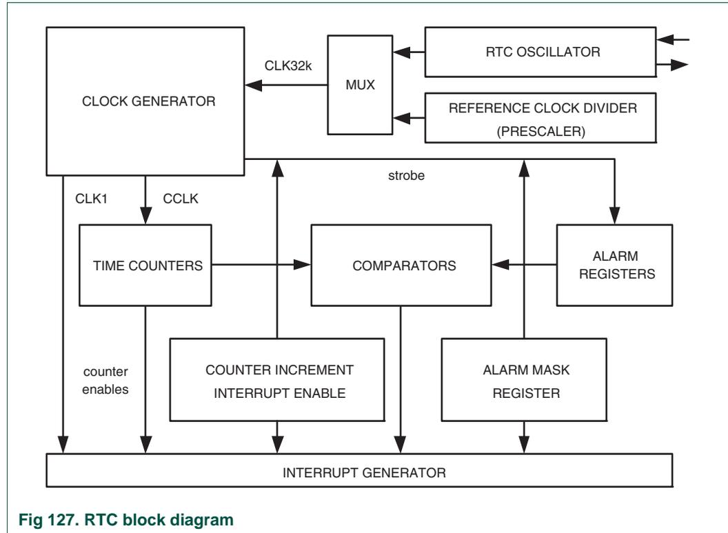
Fig 127. RTC block diagram
