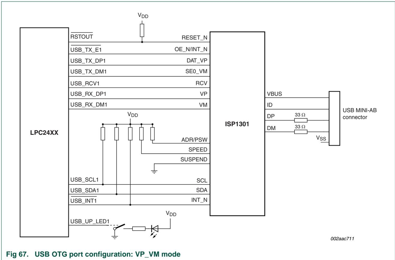
Fig 67. USB OTG port configuration: VP\_VM mode
