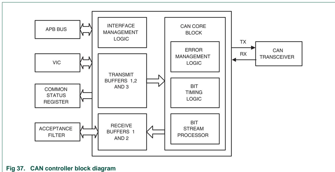
Fig 37. CAN controller block diagram
