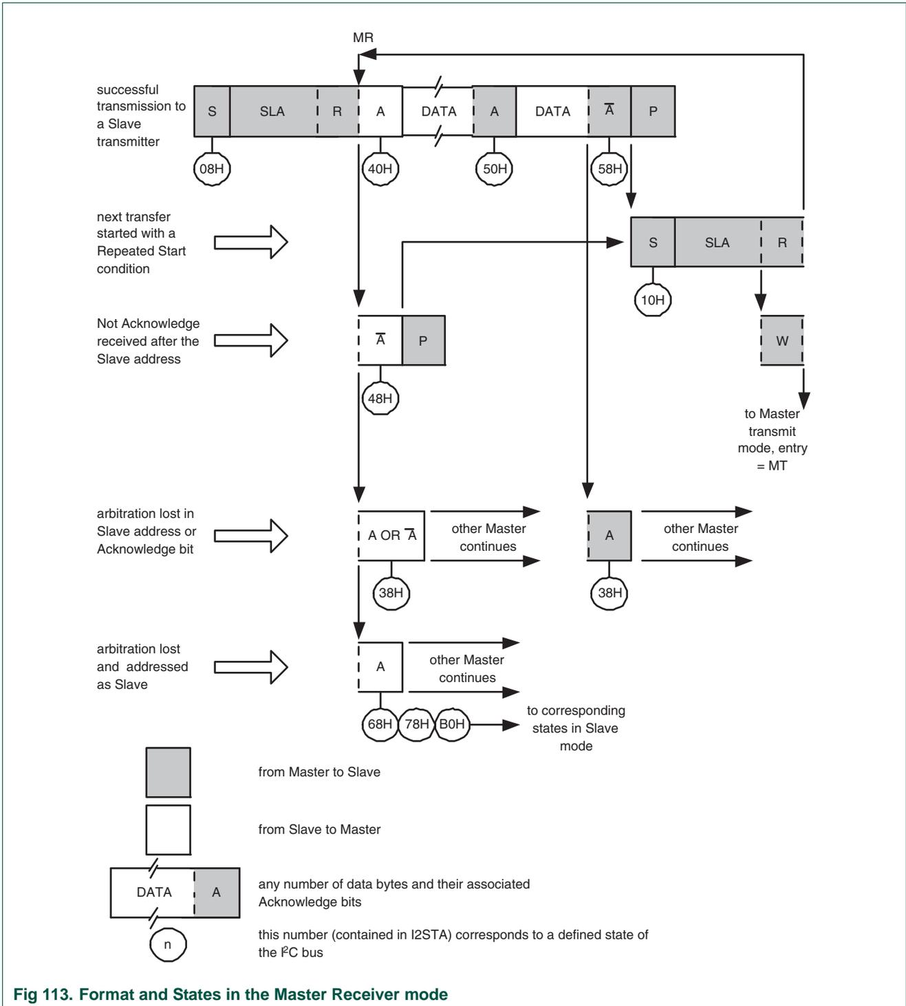
Fig 113. Format and States in the Master Receiver mode
