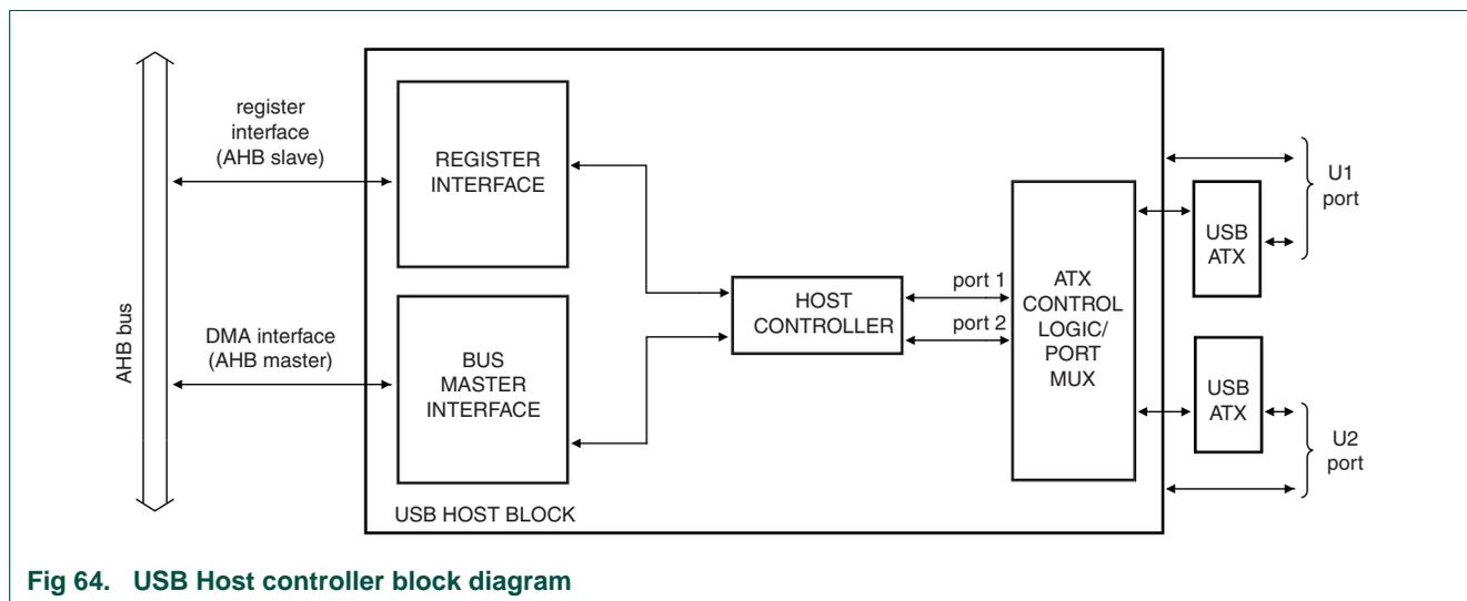
Fig 64. USB Host controller block diagram
