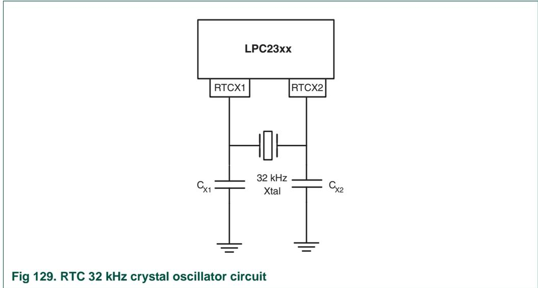
Fig 129. RTC 32 kHz crystal oscillator circuit
