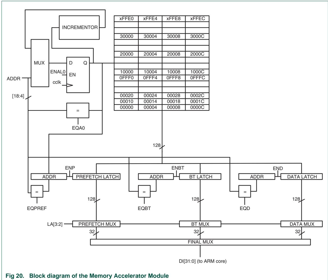
Fig 20. Block diagram of the Memory Accelerator Module
