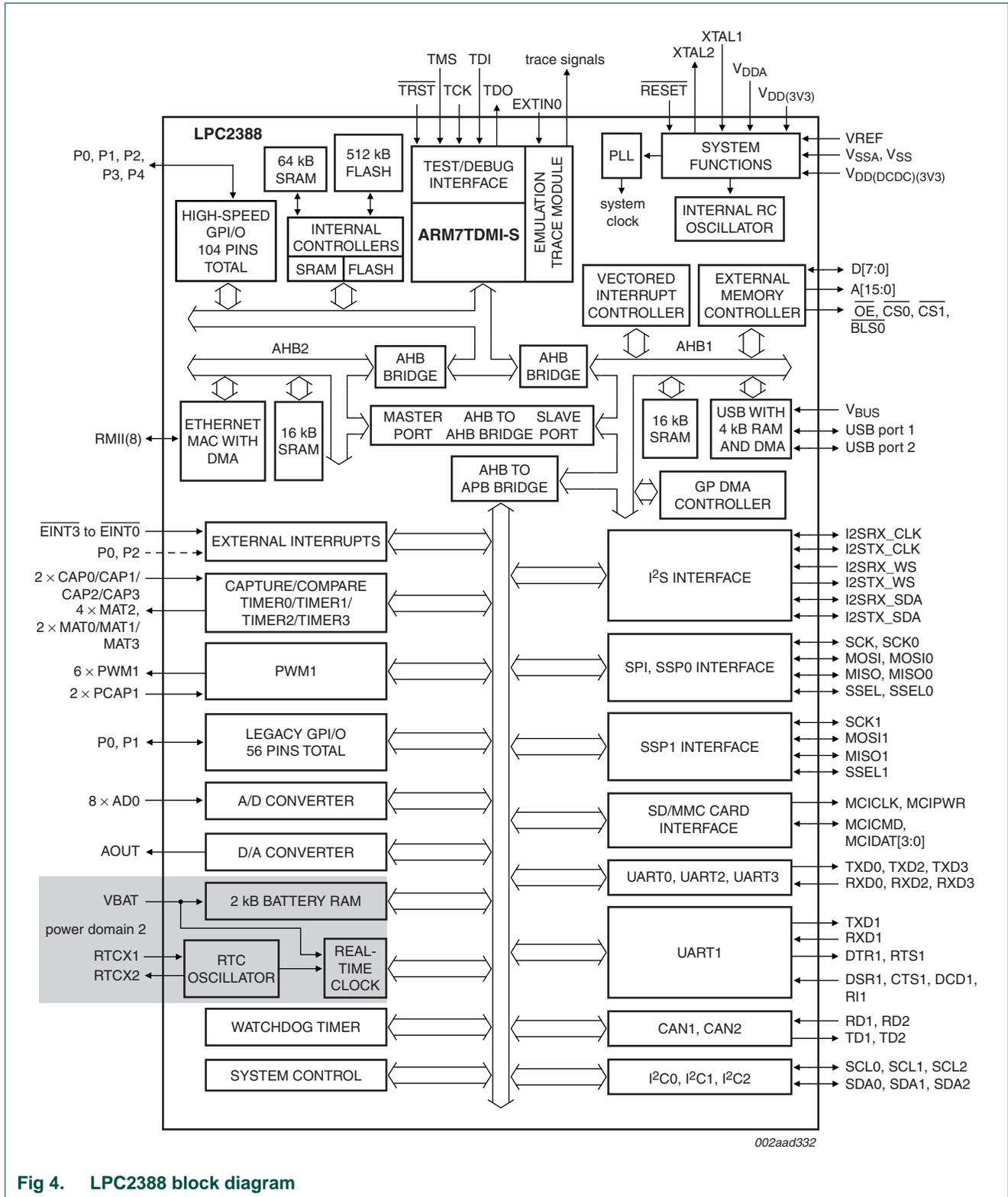
Fig 4. LPC2388 block diagram
