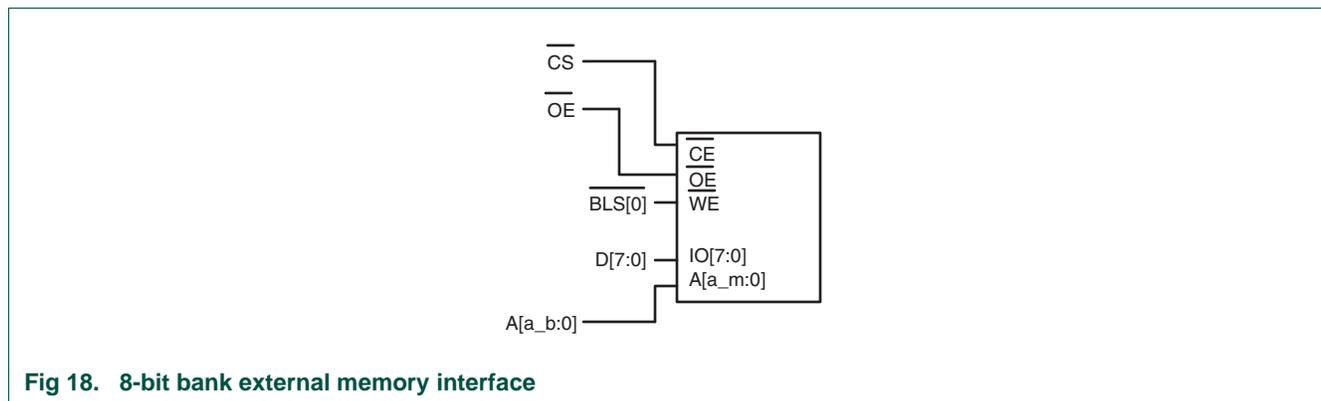
Fig 18. 8-bit bank external memory interface
