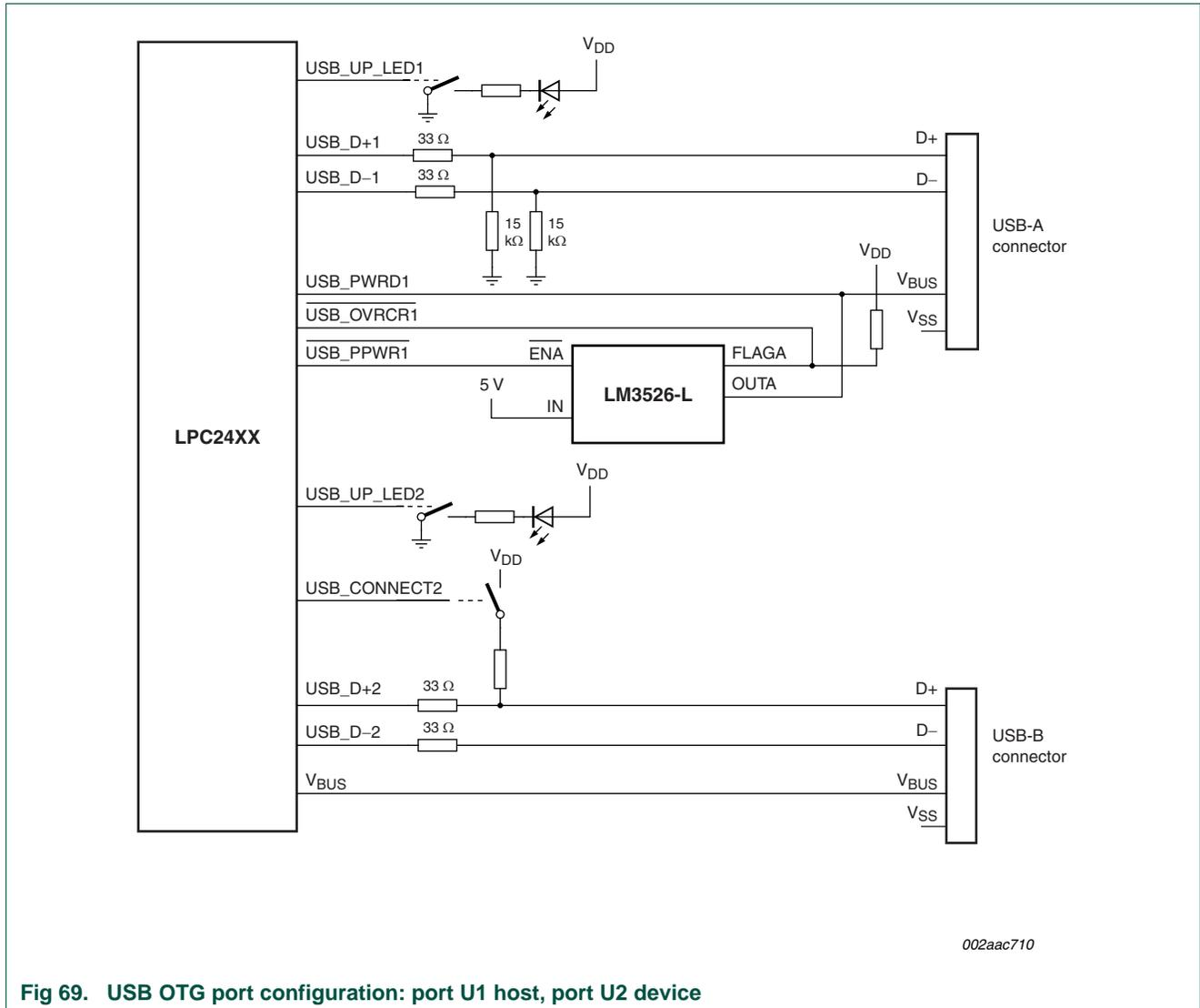
Fig 69. USB OTG port configuration: port U1 host, port U2 device
