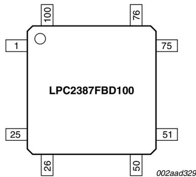
Fig 25. LPC2387 pinning LQFP100 package
