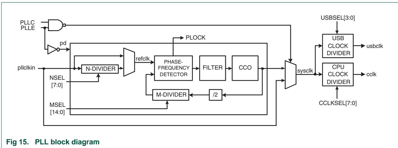
Fig 15. PLL block diagram
