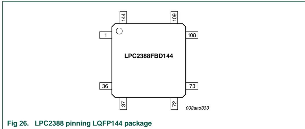
Fig 26. LPC2388 pinning LQFP144 package
