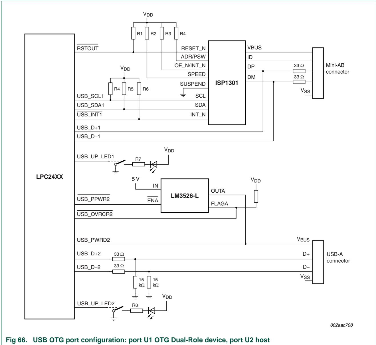
Fig 66. USB OTG port configuration: port U1 OTG Dual-Role device, port U2 host
