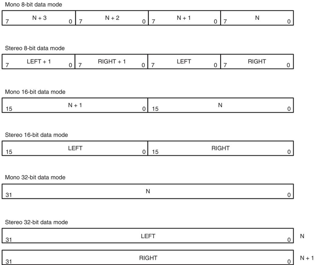
Fig 120. FIFO contents for various I<sup>2</sup>S modes
