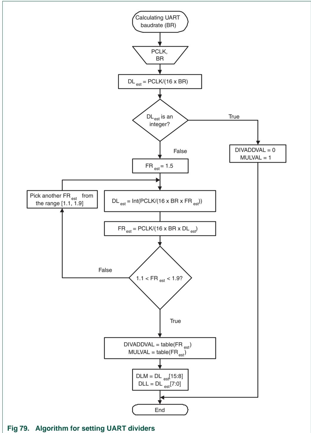
Fig 79. Algorithm for setting UART dividers
