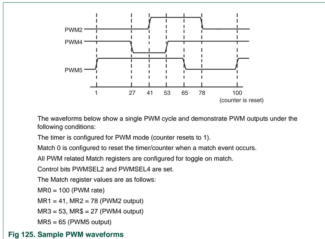
**Fig 125. Sample PWM waveforms**
