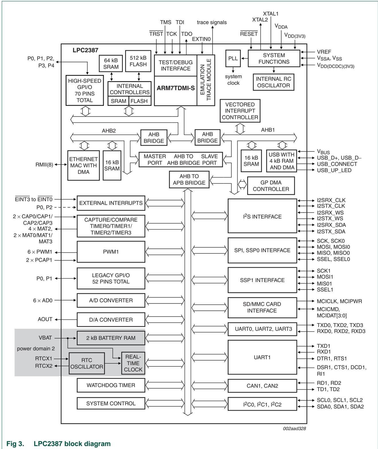
Fig 3. LPC2387 block diagram
