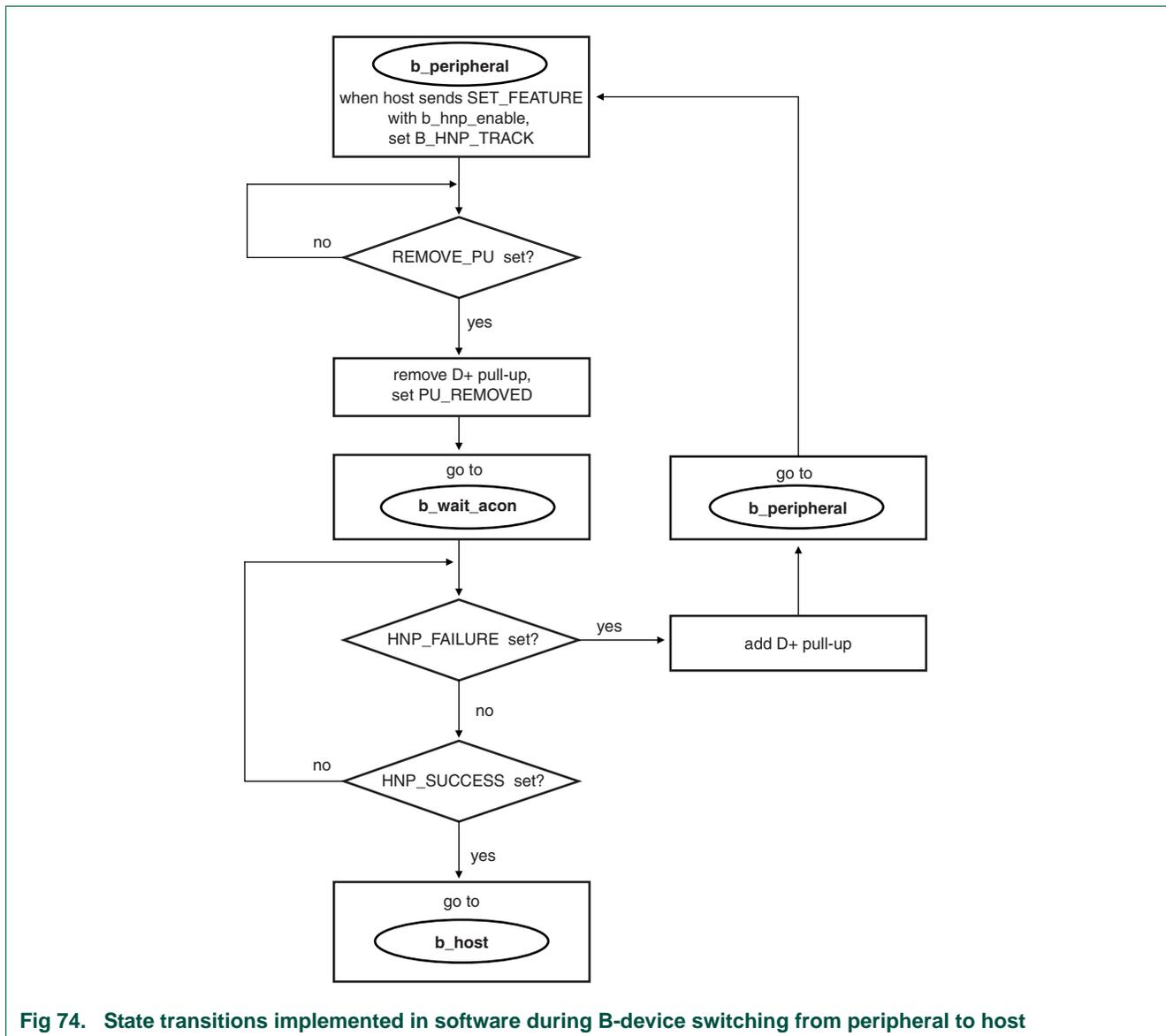
Fig 74. State transitions implemented in software during B-device switching from peripheral to host
