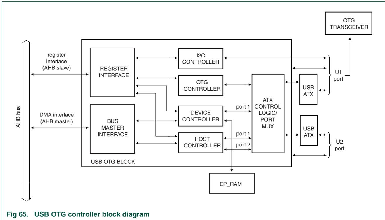
Fig 65. USB OTG controller block diagram
