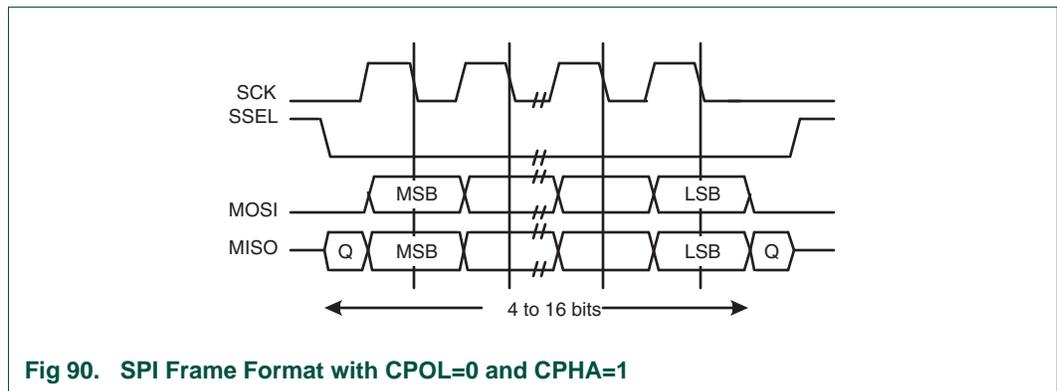
**Fig 90. SPI Frame Format with CPOL=0 and CPHA=1**
