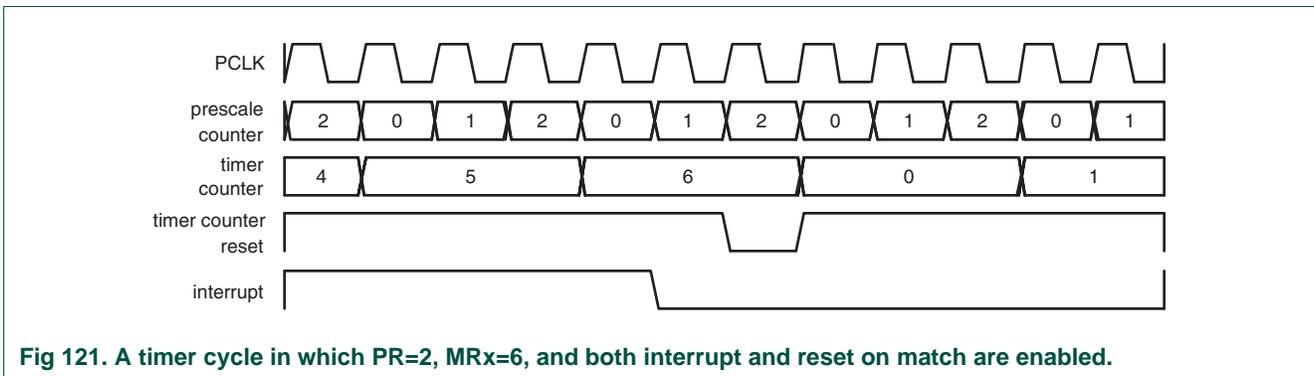
**Fig 121. A timer cycle in which PR=2, MRx=6, and both interrupt and reset on match are enabled.**
