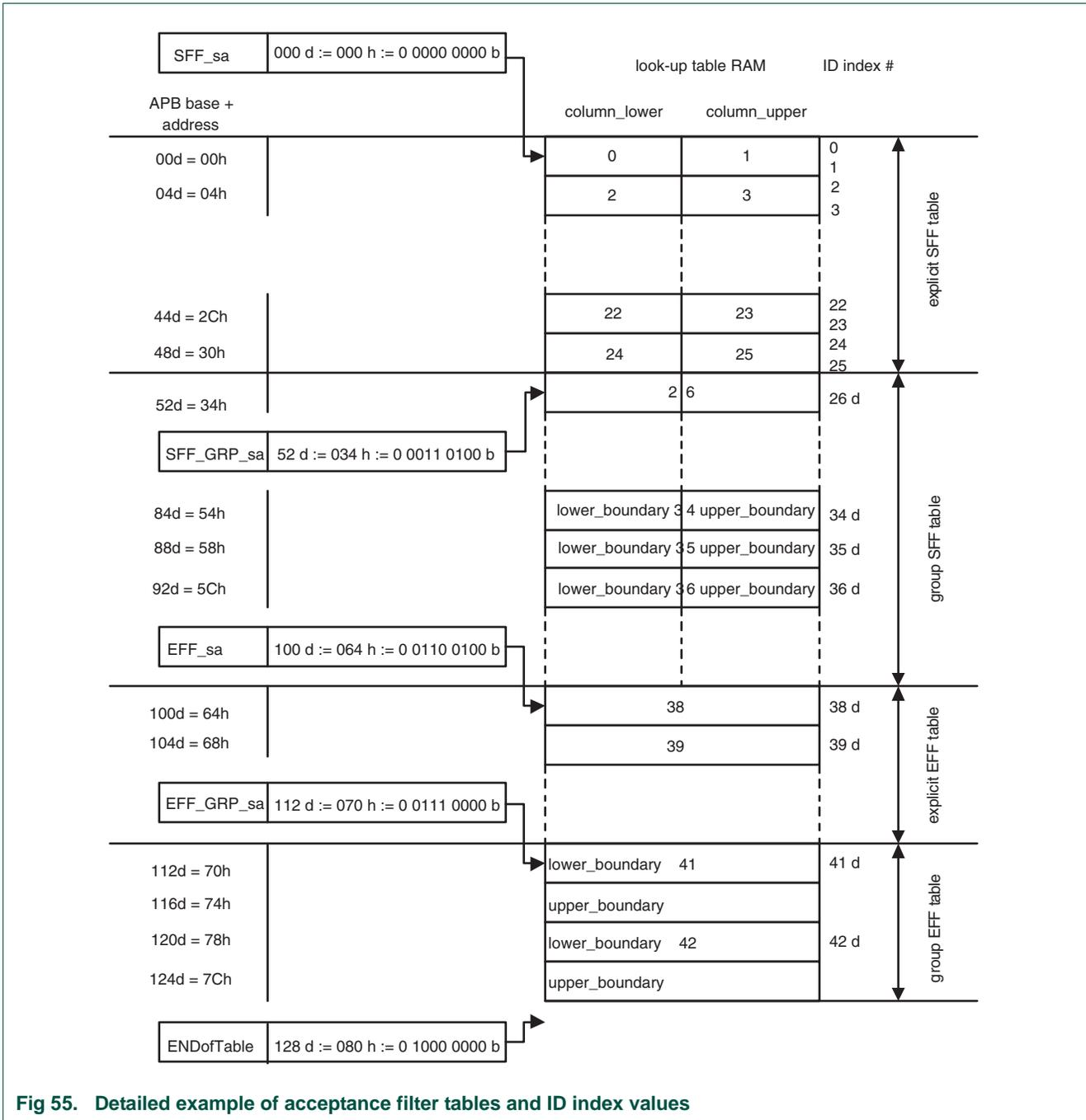
Fig 55. Detailed example of acceptance filter tables and ID index values
