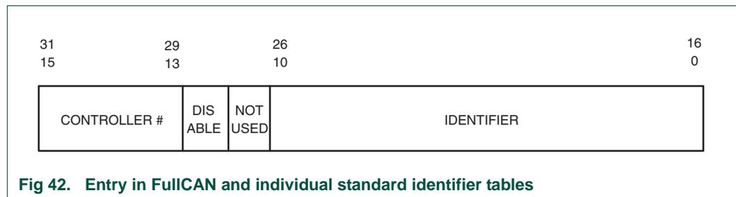
**Fig 42. Entry in FullCAN and individual standard identifier tables**
