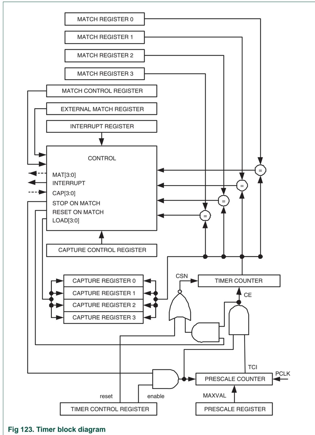
Fig 123. Timer block diagram
