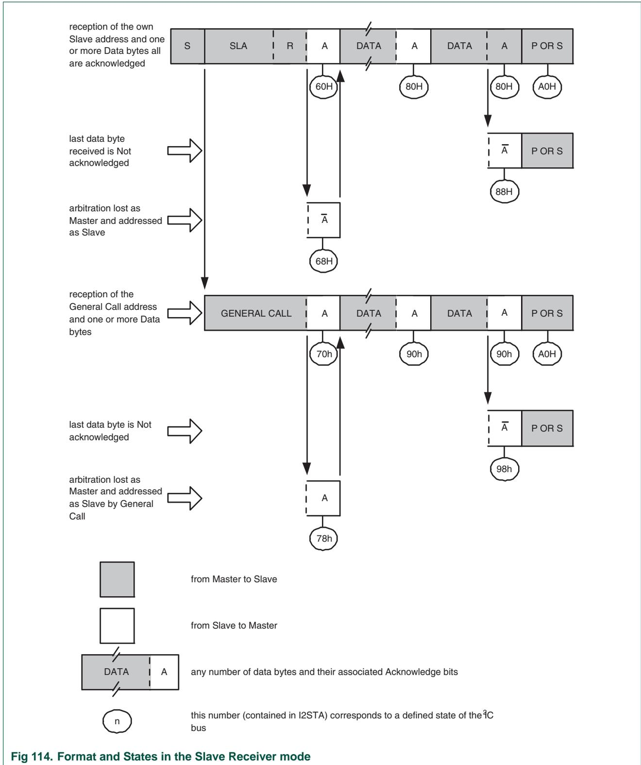
Fig 114. Format and States in the Slave Receiver mode
