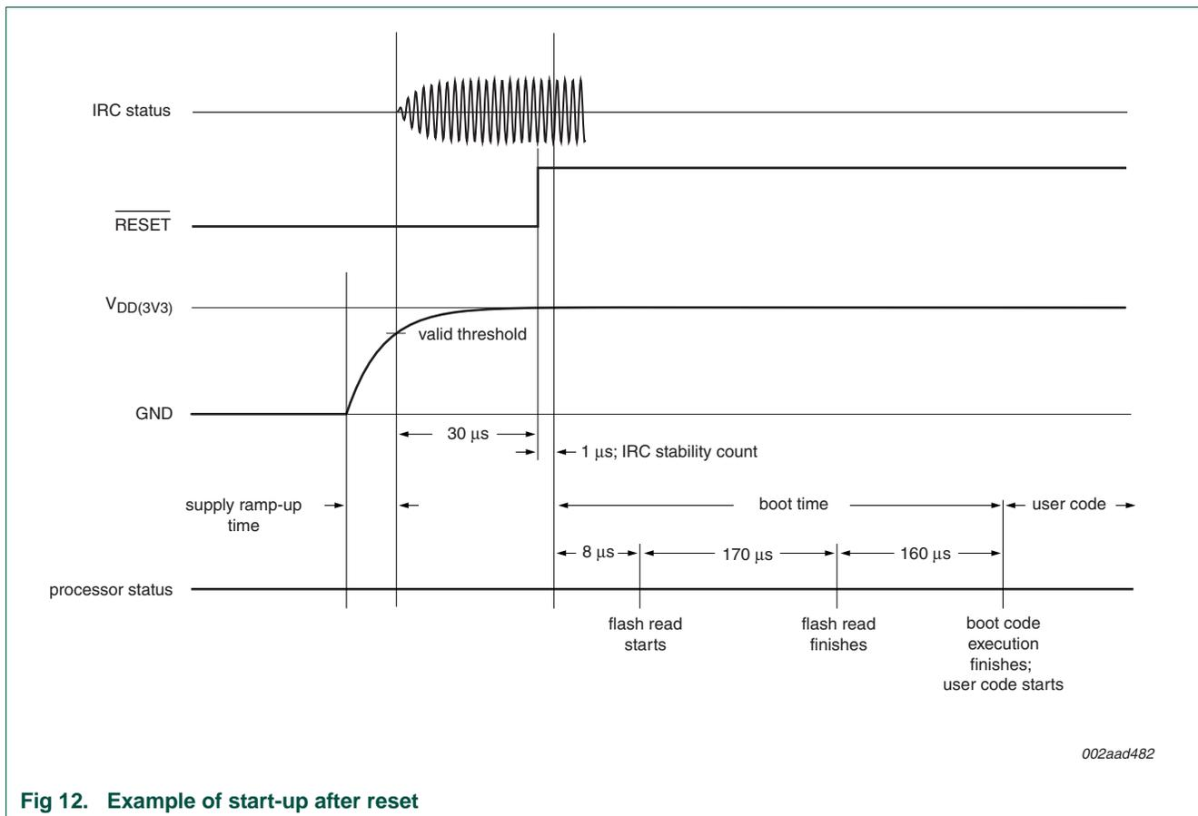
**Fig 12. Example of start-up after reset**
