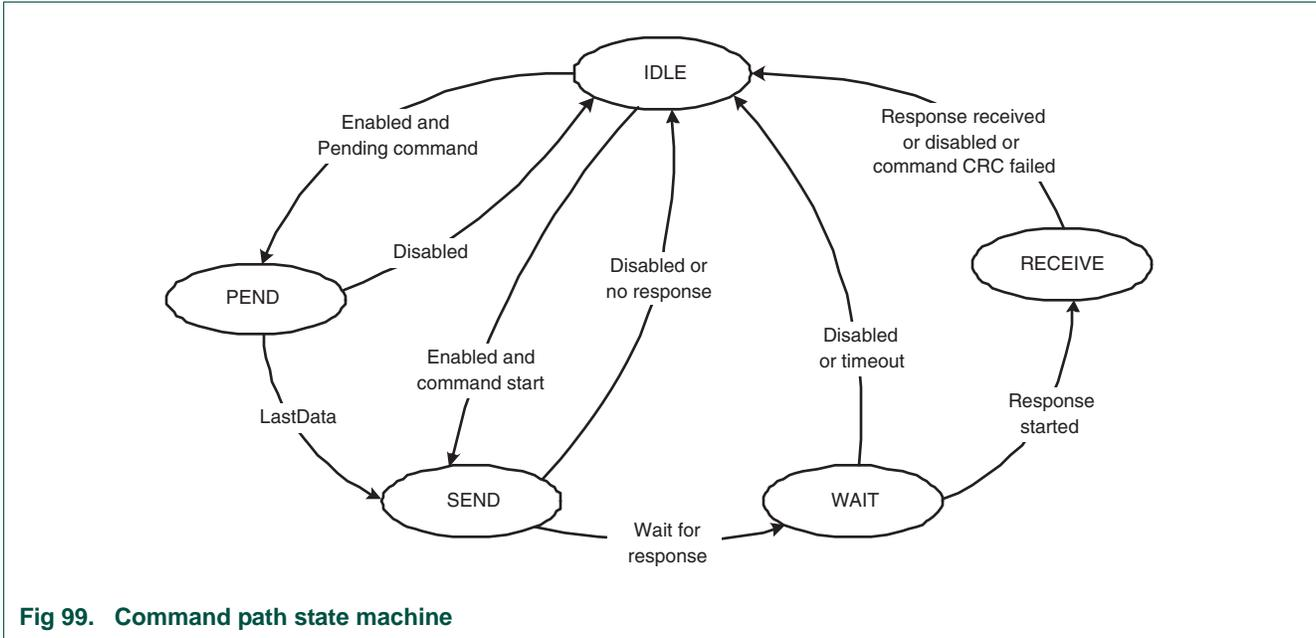
Fig 99. Command path state machine
