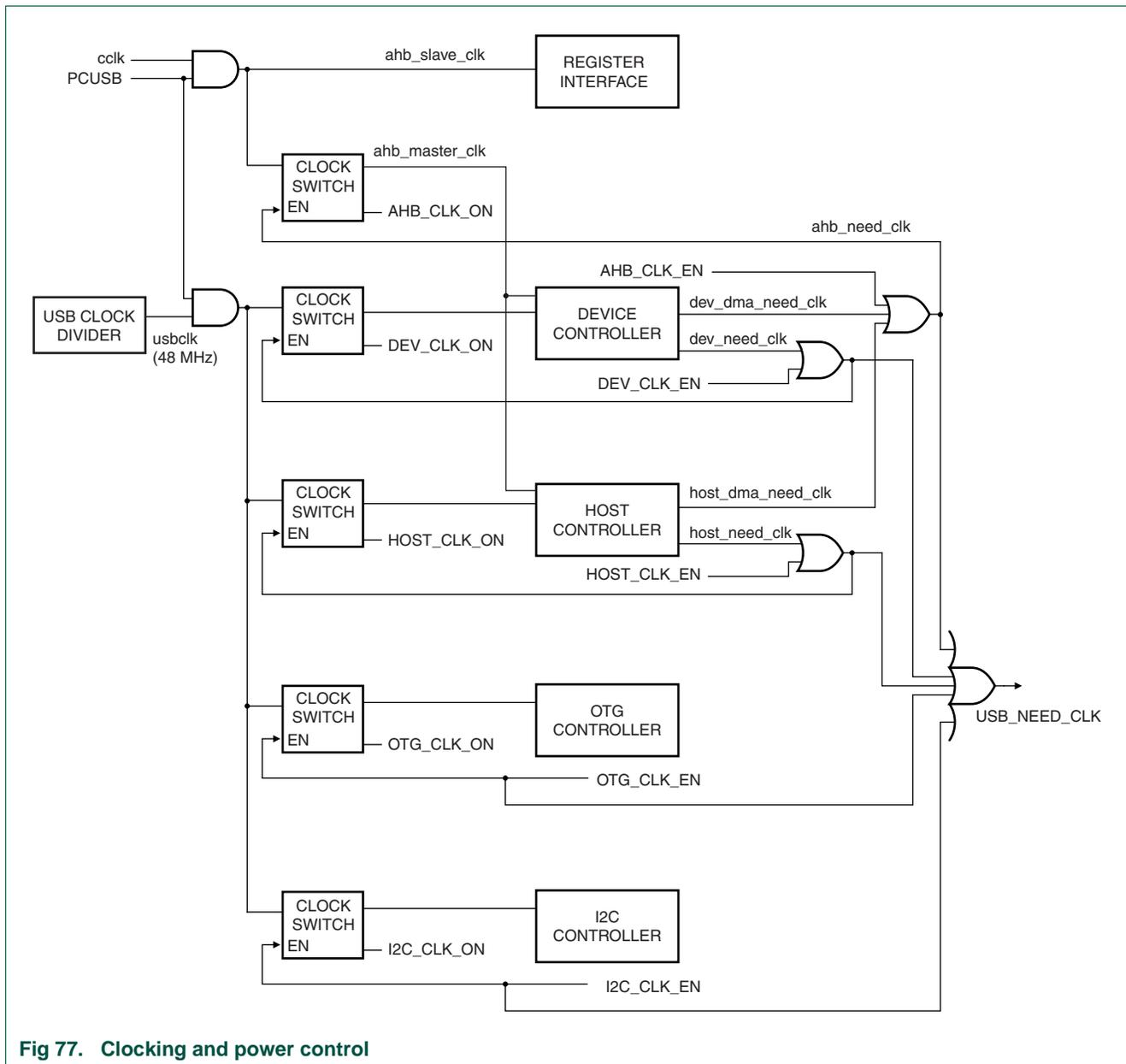
Fig 77. Clocking and power control
