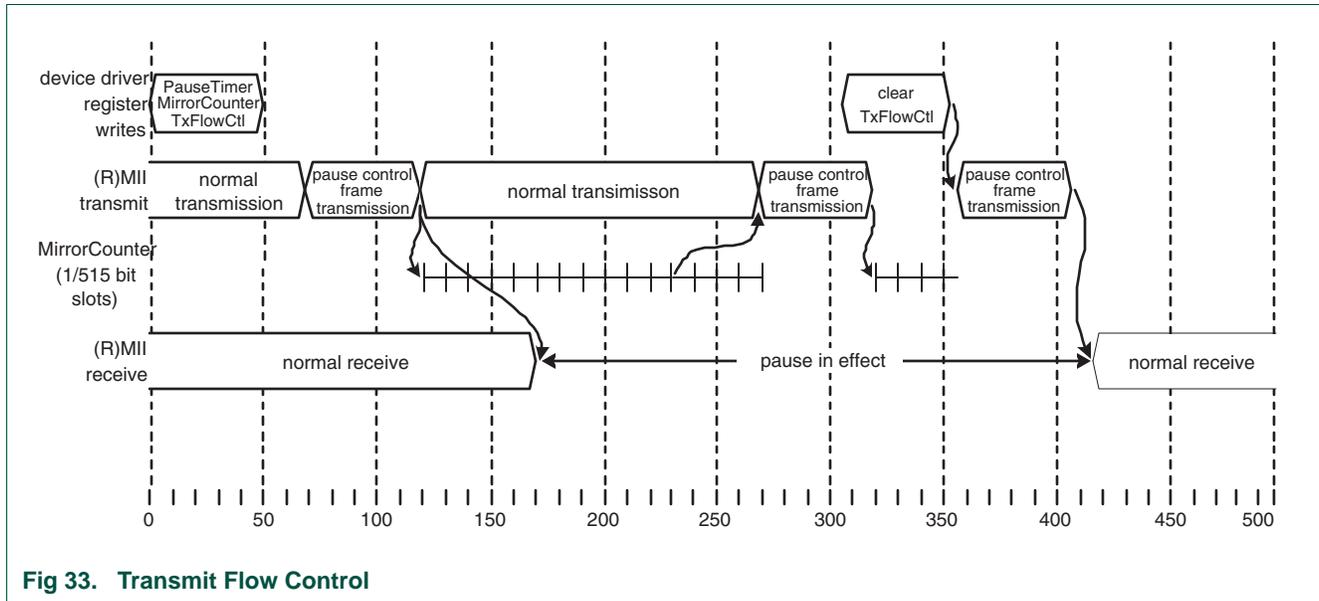
**Fig 33. Transmit Flow Control**
