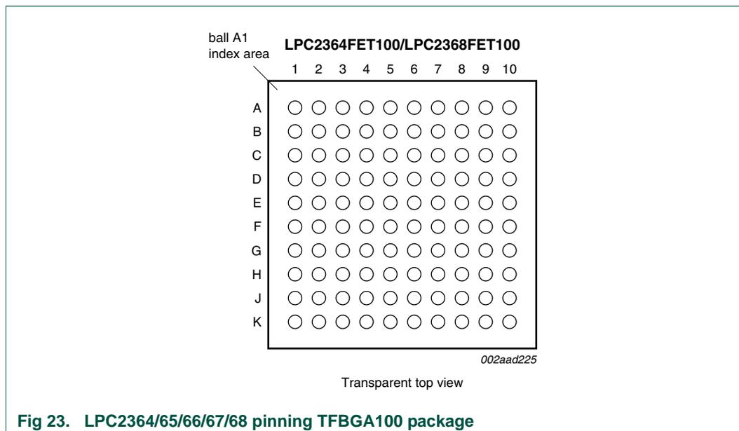
Fig 23. LPC2364/65/66/67/68 pinning TFBGA100 package
