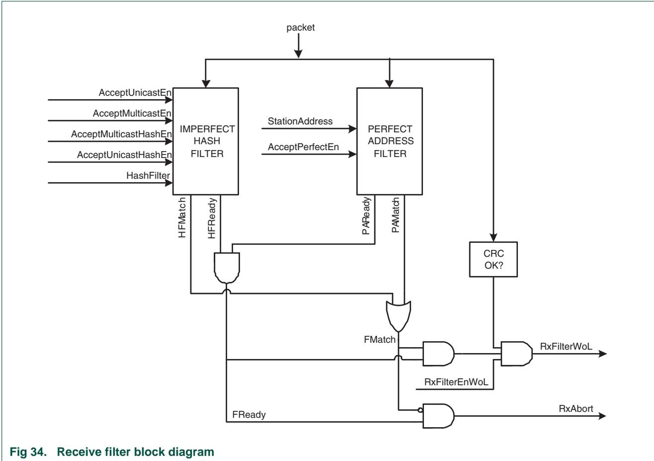
Fig 34. Receive filter block diagram
