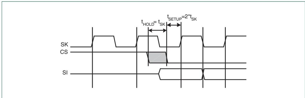
Fig 95. Microwire frame format setup and hold details
