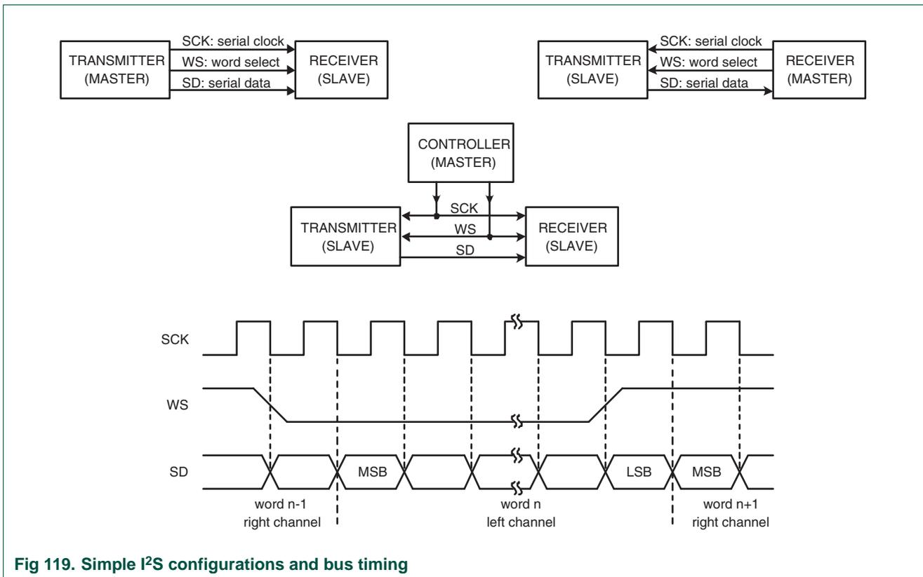
Fig 119. Simple I<sup>2</sup>S configurations and bus timing
