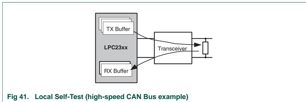
**Fig 41. Local Self-Test (high-speed CAN Bus example)**
