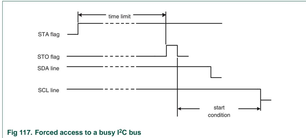
**Fig 117. Forced access to a busy I<sup>2</sup>C bus**
