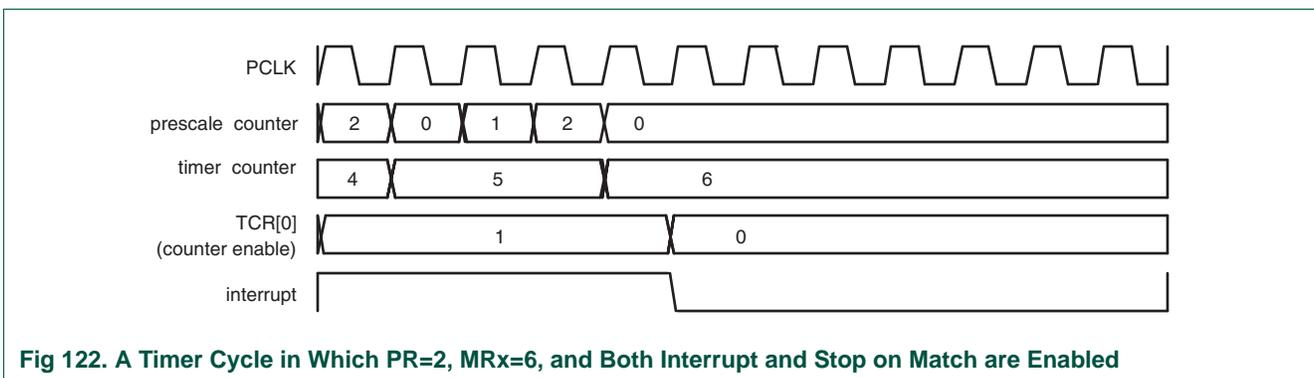
**Fig 122. A Timer Cycle in Which PR=2, MRx=6, and Both Interrupt and Stop on Match are Enabled**
