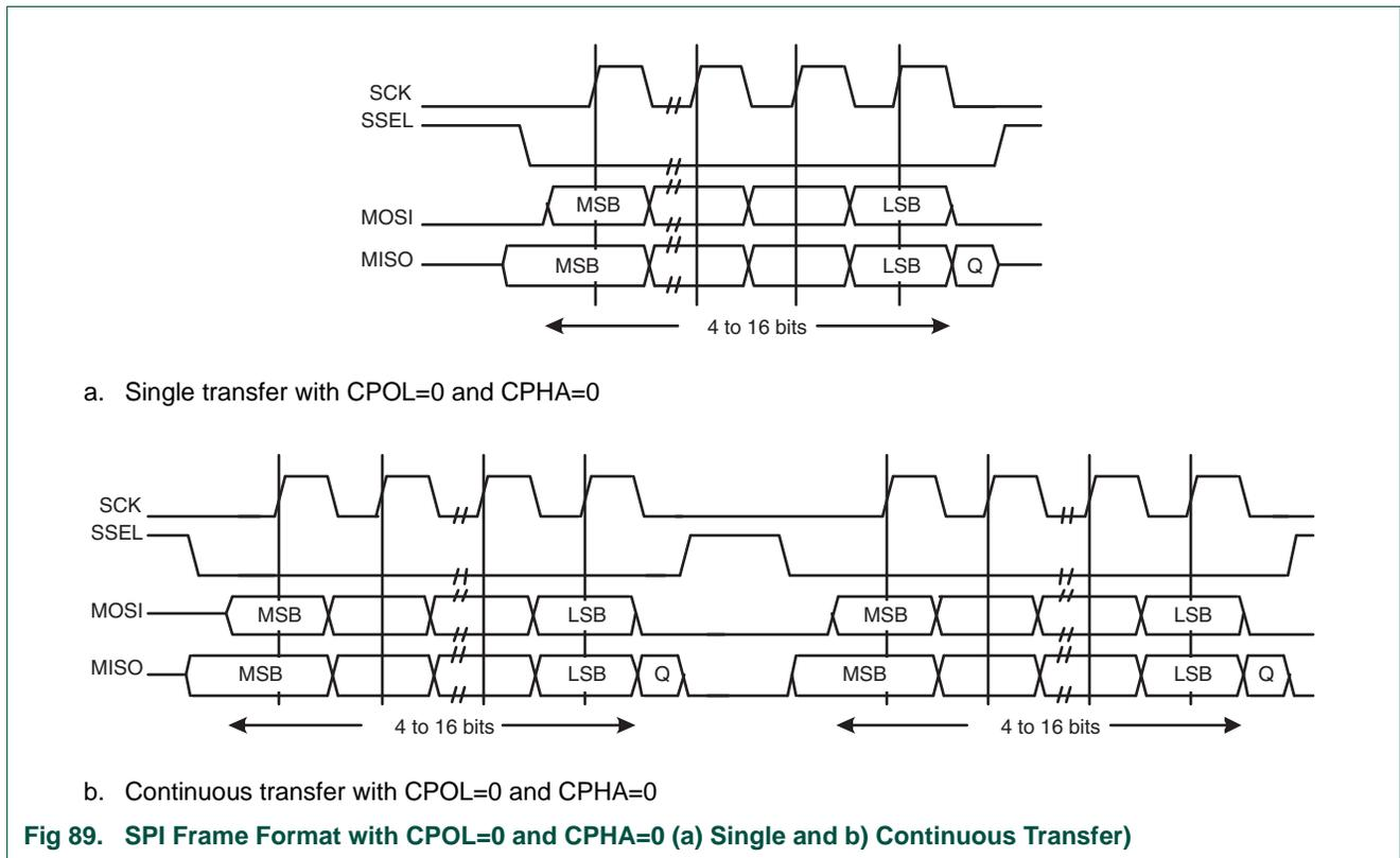
**Fig 89. SPI Frame Format with CPOL=0 and CPHA=0 (a) Single and b) Continuous Transfer)**
