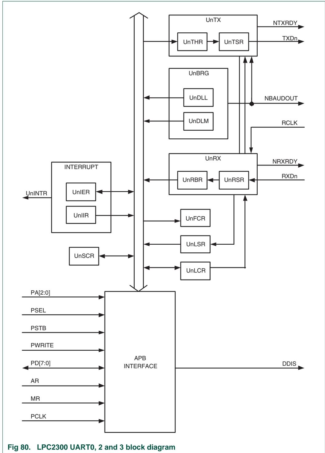
Fig 80. LPC2300 UART0, 2 and 3 block diagram
