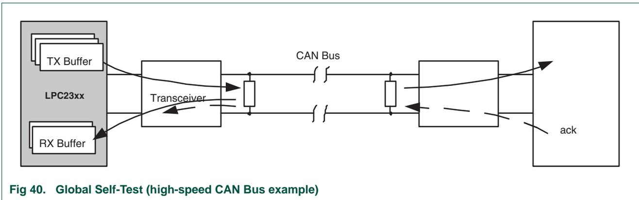
**Fig 40. Global Self-Test (high-speed CAN Bus example)**
