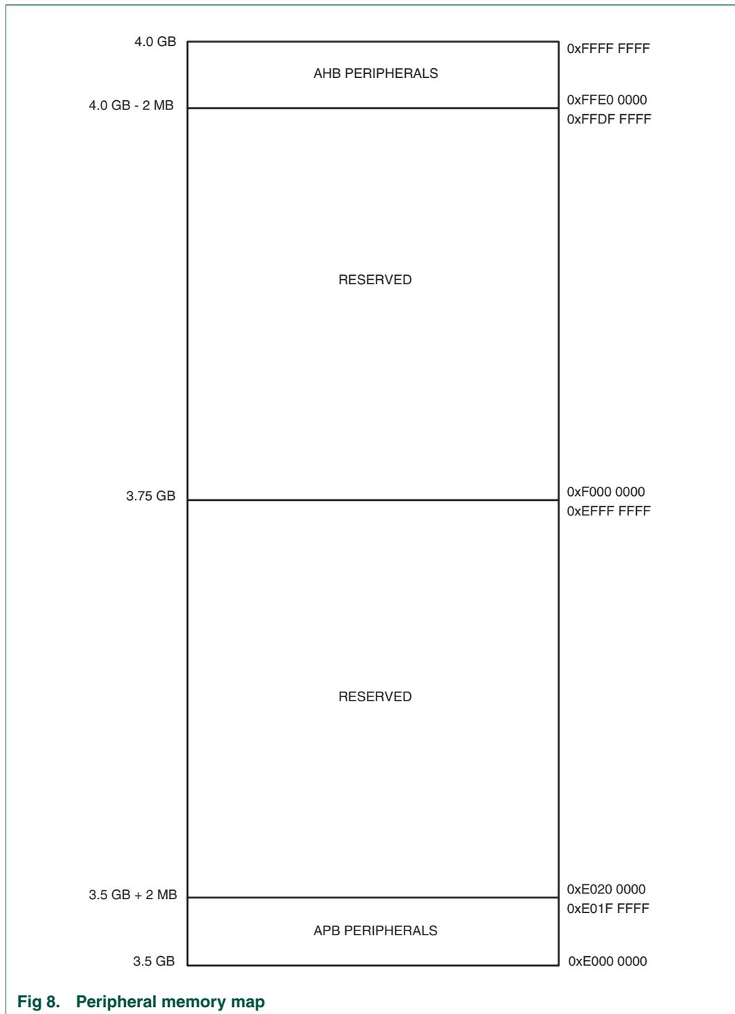
Figure 9 and Table 2-9 show different views of the peripheral address space. Both the AHB and APB peripheral areas are 2 megabyte spaces which are divided up into 128 peripherals. Each peripheral space is 16 kilobytes in size. This allows simplifying the address decoding for each peripheral.
