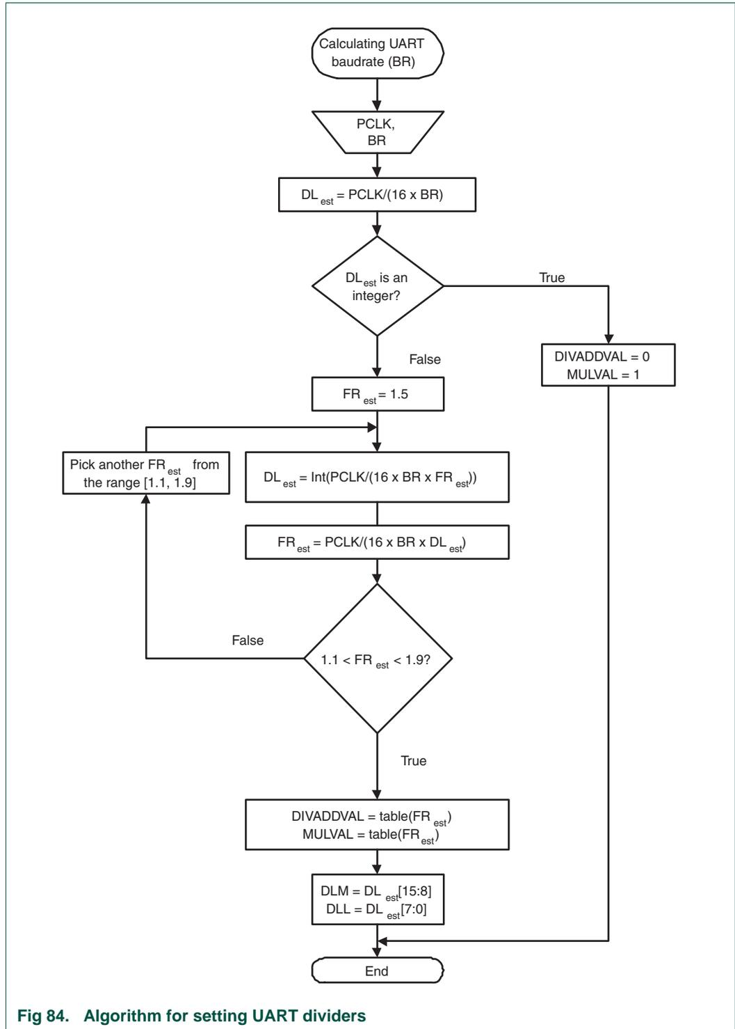
Fig 84. Algorithm for setting UART dividers
