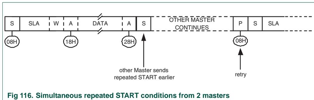
Fig 116. Simultaneous repeated START conditions from 2 masters
