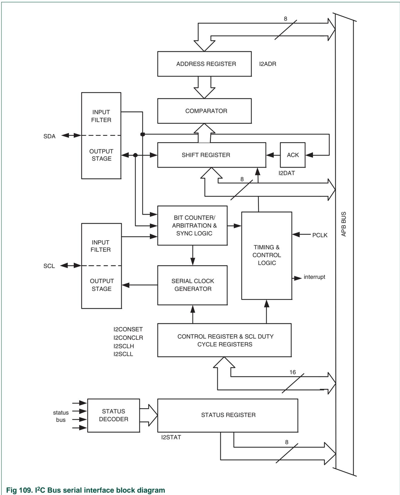
Fig 109. I<sup>2</sup>C Bus serial interface block diagram
