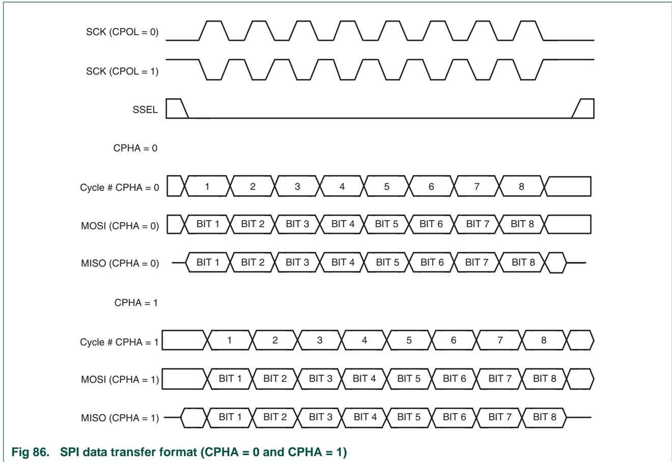
**Fig 86. SPI data transfer format (CPHA = 0 and CPHA = 1)**
