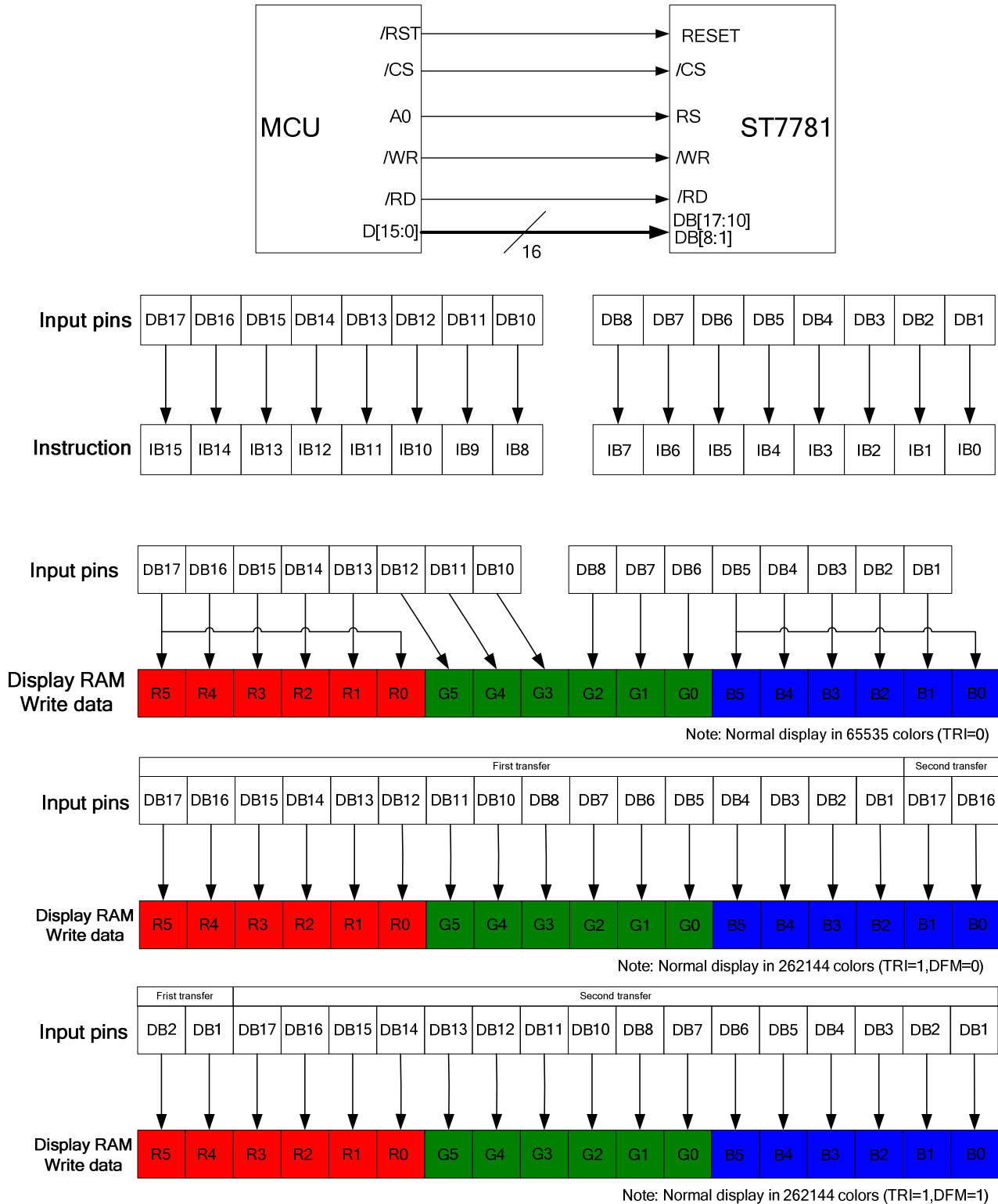
Fig. 9.4 8080-16 bits Interface Data Format (Command Write/Display RAM Write)
